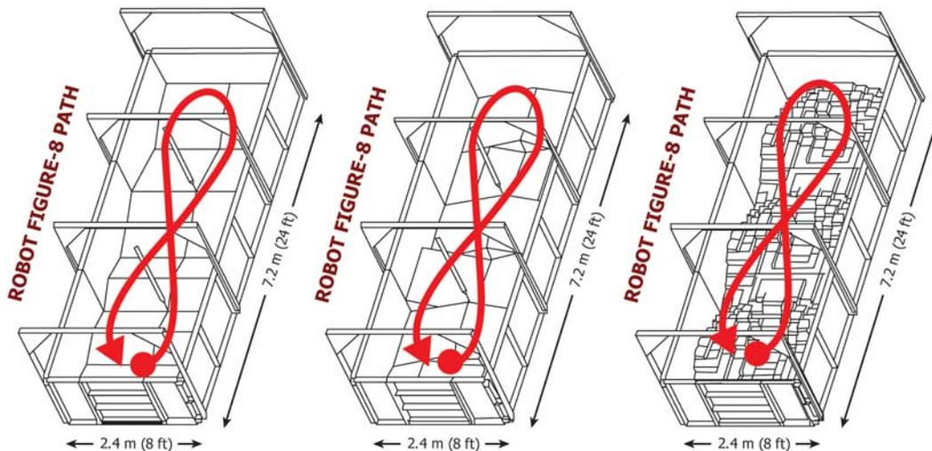
FIG. 2 Three Confined Area Terrain Apparatuses in the Mobility Test Suite with Increasing Complexity; The Continuous Pitch/Roll Ramps Terrain is Shown on the Left. The Crossing Pitch/Roll Ramps is Shown at the Center. The Symmetric Stepfields Terrain is Shown on the Right.
