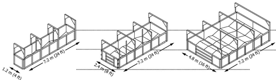
FIG. 1 Mobility: Confined Area Terrains: Continuous Pitch/Roll Ramps Apparatuses
