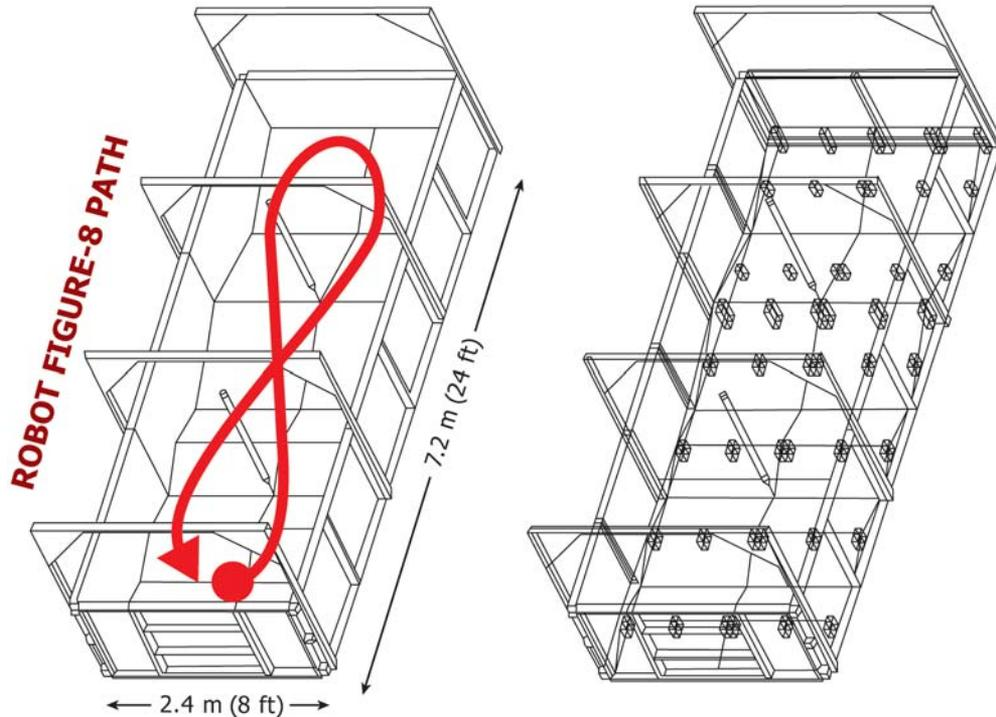
FIG. 3 Mobility: Confined Area Terrains: Continuous Pitch/Roll Ramps Apparatuses (Perspective View)
