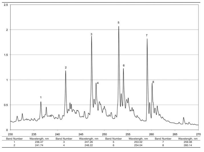
Instrument: Cary 5000 Scanning Speed: 0.6 nm/min Spectral Bandwidth: 0.1 nm Spectral Data Interval: 0.02 nm
