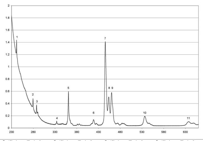
Wavelength, nm Band Number Wavelength, nm **Band Number** Wavelength, nm Band Number Band Number Wavelength, nm 241.64 333.86 445.67 10 536.27 2 279.38 5 360.92 8 453.62 11 637.69 3 287.55 6 418.66 9 460.21
