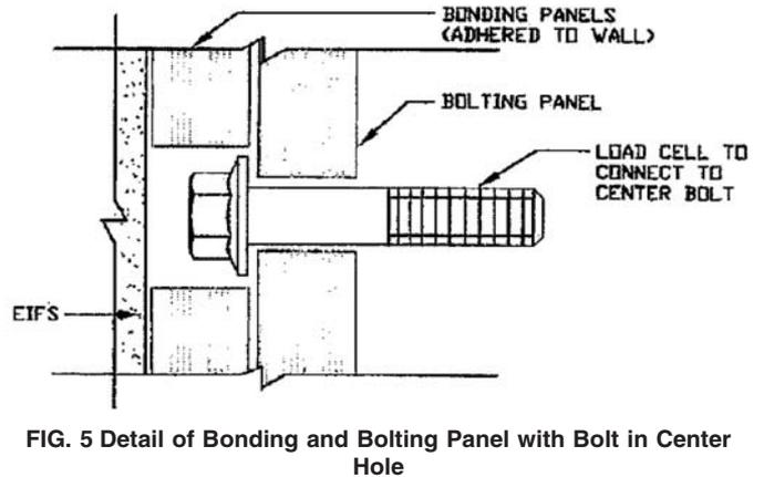
FIG. 5 Detail of Bonding and Bolting Panel with Bolt in Center Hole
