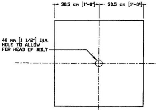
FIG. 2 Bonding panel
