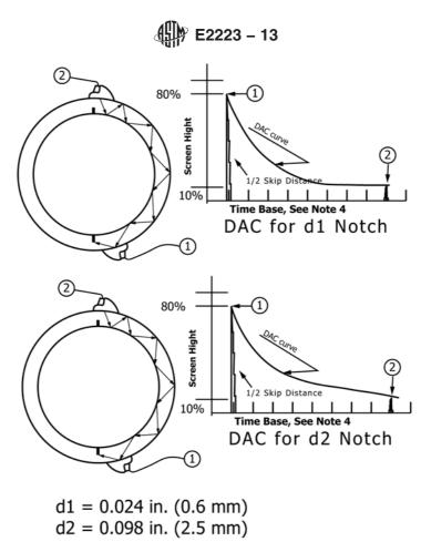
Note 1—Time base shall be sufficient in length to display the cylinder's circumference.
