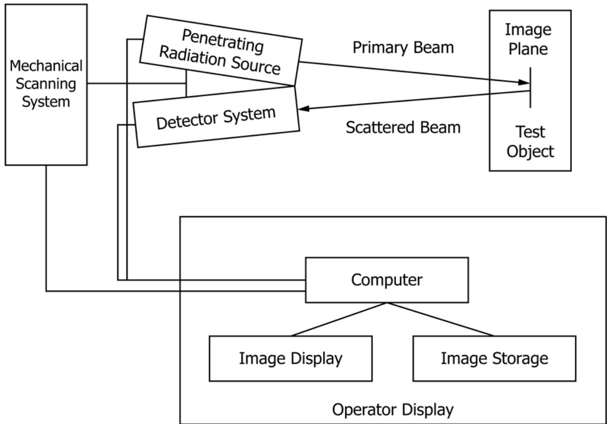
FIG. 8 Typical CST System Block Diagram
