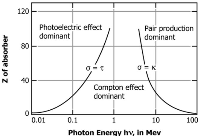
**FIG. 1 Relationship Between Photoelectric, Compton, and Pair Production Effects**
