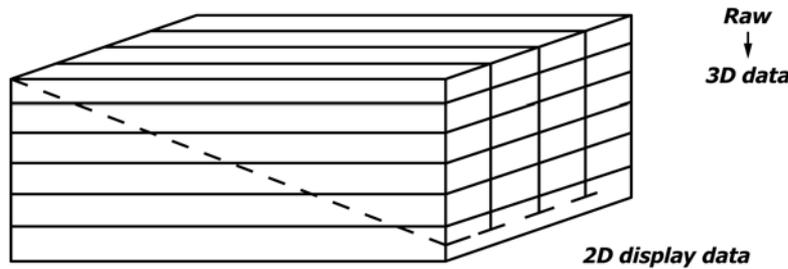
FIG. 11 Tomographic Slice Images May be Generated at Any Angle With Respect to the Original Slice Images
