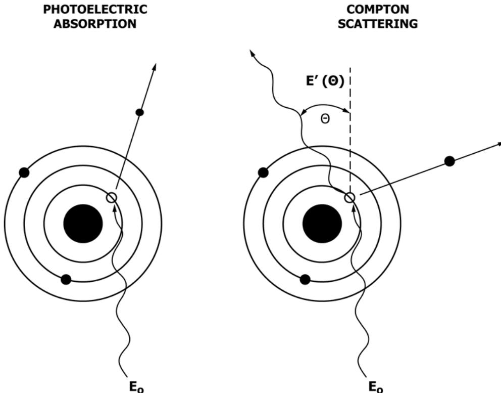
FIG. 2 Principles of Photoelectric Absorption and Compton Scattering
