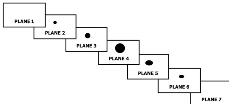
FIG. 7 Simulated CST Image Display of a Homogenous Examination Object Containing a Void
