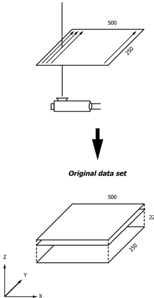
FIG. 6 Typical CST Imaging Scan Plan
