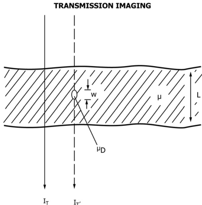
FIG. 4 Schematic Representation of the Transmitted Beam Imaging System Technique
