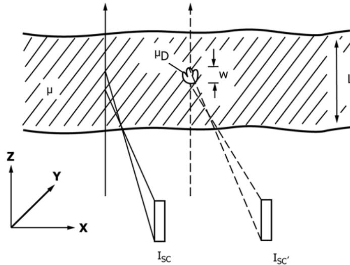
FIG. 5 Schematic Representation of the Compton Scatter Tomography Technique
