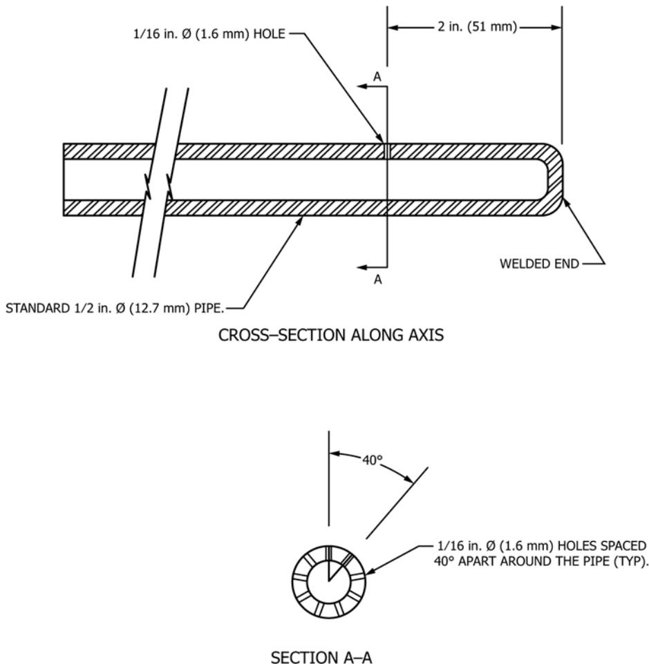
FIG. 2 Furnace Pressure Probe 2
