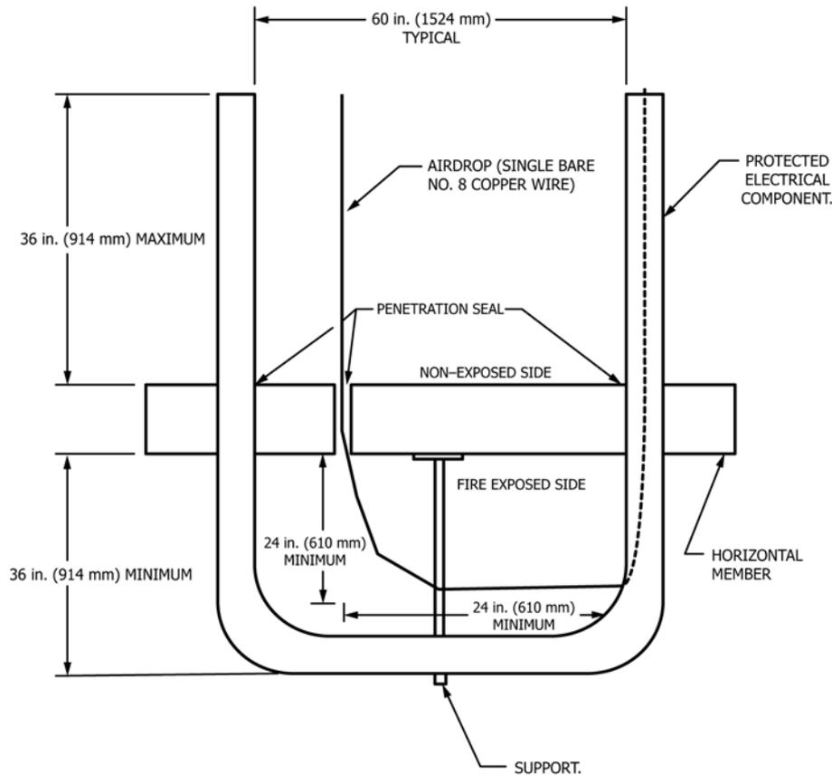
FIG. 6 Vertical and Horizontal Air Drop Assembly
