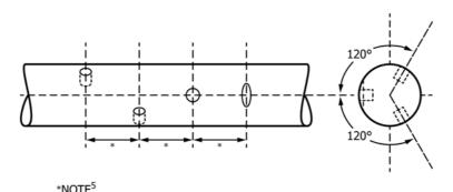
Note 1—A suggested length between discontinuities is 2 in. (51 mm). However, this space should be sufficient to provide signal resolution adequate for interpretation. The speed of the reference standard through the test coil is not critical, but a range from 5 to 150 ft/min (1.5 to 45.72 m/min) is recommended.
