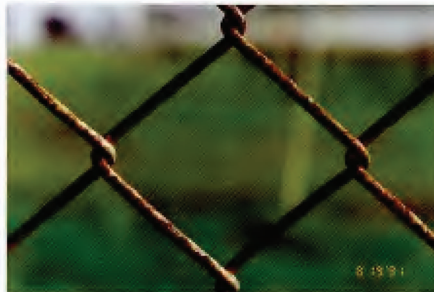
FIG. 19. Specimen 34 – Zinc Electroplated Chain Link Fabric. Original coating weight: 1.53 oz/ft 2 (467 g/m 2 ). Exposure site: Kure Beach, NC (800-ft site). 30-year condition of links (see Table 13): 60R, 35wc, 5G.
