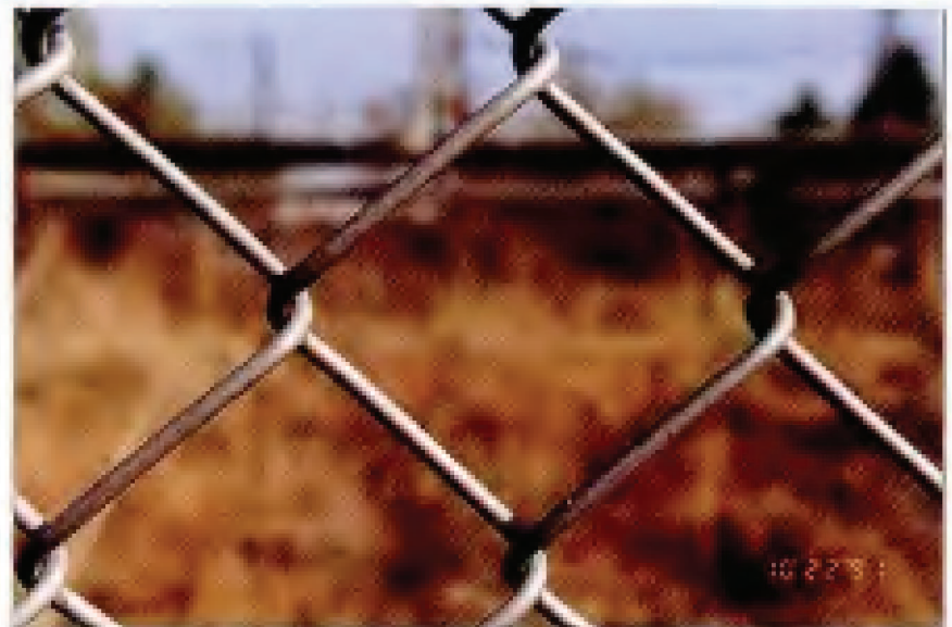
FIG. 33. Specimen 36 – Hot-Dip Aluminized Chain Link Fabric. Original coating weight: 0.57 oz/ft 2 (174 g/m 2 ). Exposure site: Manhattan, KS. 30-year condition of links (see Table 13): 50M, 50G.
