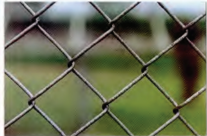
FIG. 53. Specimen 38 – Hot-Dip Aluminized Chain Link Fabric. Original coating weight: 0.54 oz/ft 2 (165 g/m 2 ). Exposure site: State College, PA. 30-year condition of links (see Table 13): 15PPR, 5Y, 80G.
