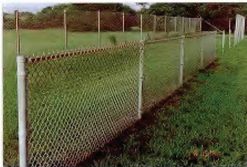
FIG. 3. Overall View of the Kure Beach, NC 800-ft Test Site illustrates the mounting of the chain link fabric test specimens.
