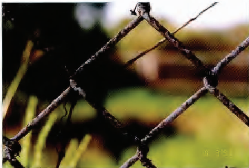
FIG. 11. Specimen 33 – Hot-dip Galvanized Chain Link Fabric. Original coating weight: 2.81 oz/ft 2 (857 g/m 2 ). Exposure site: Brazos River, TX. 30-year condition of links (see Table 13): 60R, 40wc.
