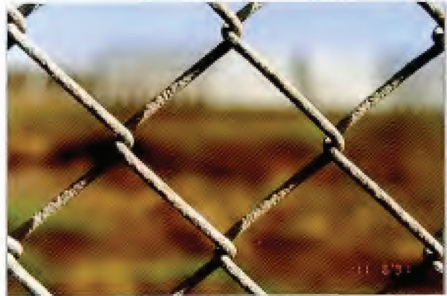
FIG. 28. Specimen 35 – Zinc Electroplated Chain Link Fabric. Original coating weight: 2.23 oz/ft 2 (680 g/m 2 ). Exposure site: Point Reyes, CA. 30-year condition of links (see Table 13): 5R, 75wc, 20G.
