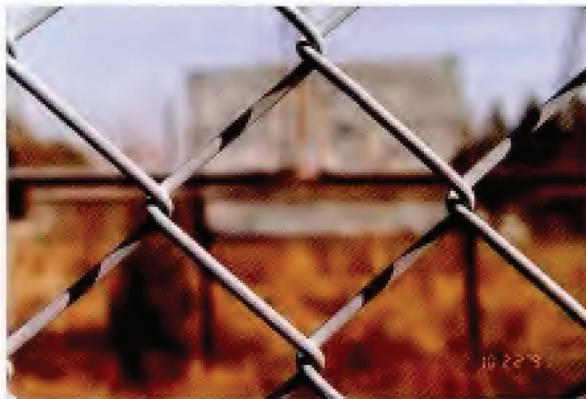
FIG. 26. Specimen 35 – Zinc Electroplated Chain Link Fabric. Original coating weight: 2.23 oz/ft 2 (680 g/m 2 ). Exposure site: Manhattan, KS. 30-year condition of links (see Table 13): 100G.
