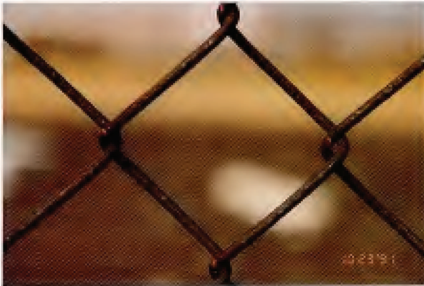
FIG. 8. Specimen 32 – Hot-dip Galvanized Chain Link Fabric. Original coating weight: 1.77 oz/ft 2 (540 g/m 2 ). Exposure site: Newark-Kearny, NJ. 30-year condition of links (see Table 13): 100R.
