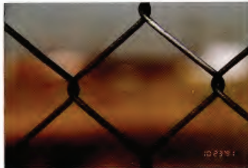
FIG. 43. Specimen 37 – Hot-Dip Aluminized Chain Link Fabric. Note: This is same specimen as illustrated in Fig. 42, with black corrosion product removed on one straight wire segment to illustrate that aluminum coating is still intact.
