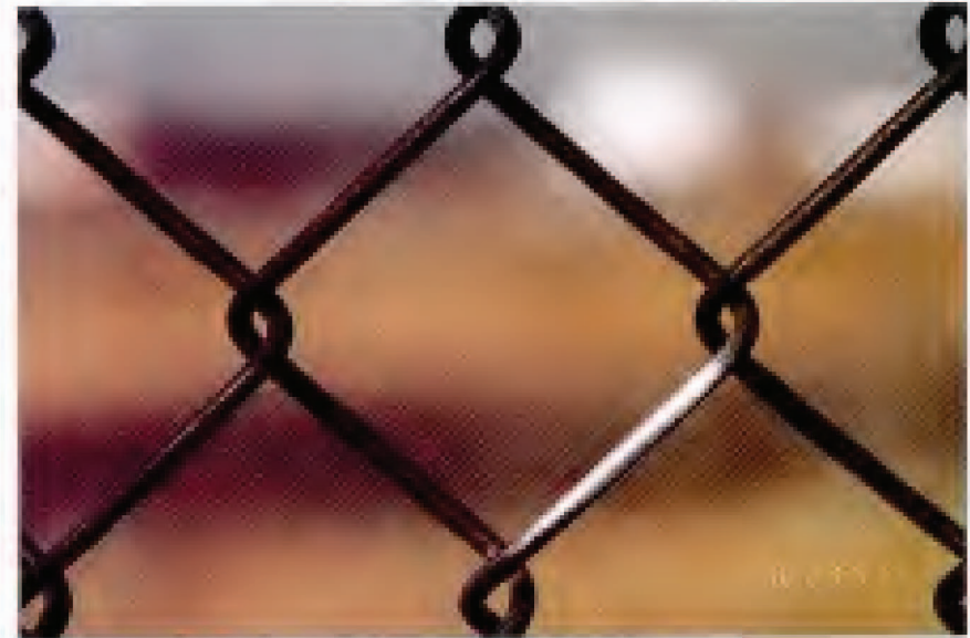
FIG. 51. Specimen 38 – Hot-Dip Aluminized Chain Link Fabric. Note: This is same specimen as illustrated in Fig. 50, with black corrosion product removed on one straight wire segment to illustrate that aluminum coating is still intact.
