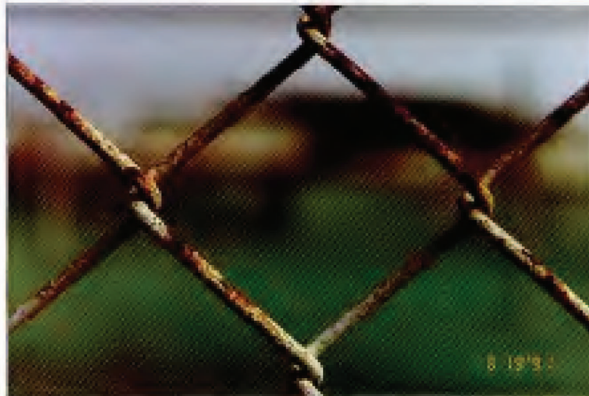
FIG. 25. Specimen 35 – Zinc Electroplated Chain Link Fabric. Original coating weight: 2.23 oz/ft 2 (680 g/m 2 ). Exposure site: Kure Beach, NC (800-ft site). 30-year condition of links (see Table 13): 30R, 60wc, 10G.
