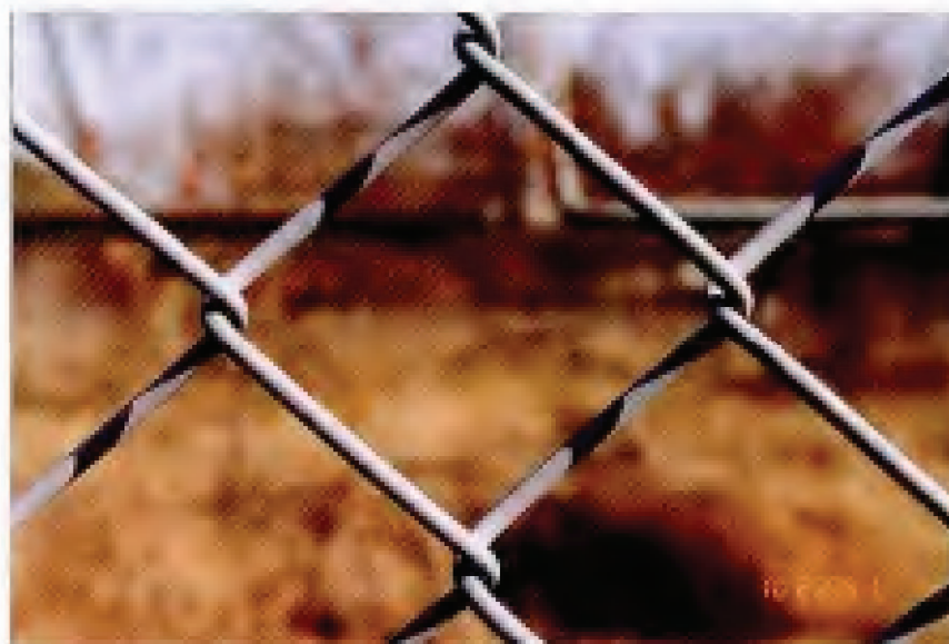
FIG. 20. Specimen 34 – Zinc Electroplated Chain Link Fabric. Original coating weight: 1.53 oz/ft 2 (467 g/m 2 ). Exposure site: Manhattan, KS. 30-year condition of links (see Table 13): 100G.
