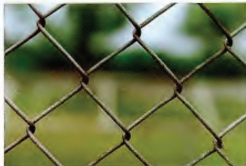
FIG. 45. Specimen 37 – Hot-Dip Aluminized Chain Link Fabric. Original coating weight: 0.44 oz/ft 2 (134 g/m 2 ). Exposure site: State College, PA. 30-year condition of links (see Table 13): 15PPR, 15Y, 70G.
