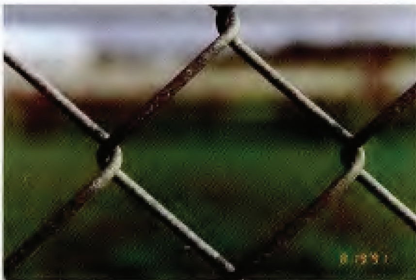
FIG. 48. Specimen 38 – Hot-Dip Aluminized Chain Link Fabric. Original coating weight: 0.54 oz/ft 2 (165 g/m 2 ). Exposure site: Kure Beach, NC (800 ft site). 30-year condition of links (see Table 13): trR, trY, 40wc, 50G, 10M.
