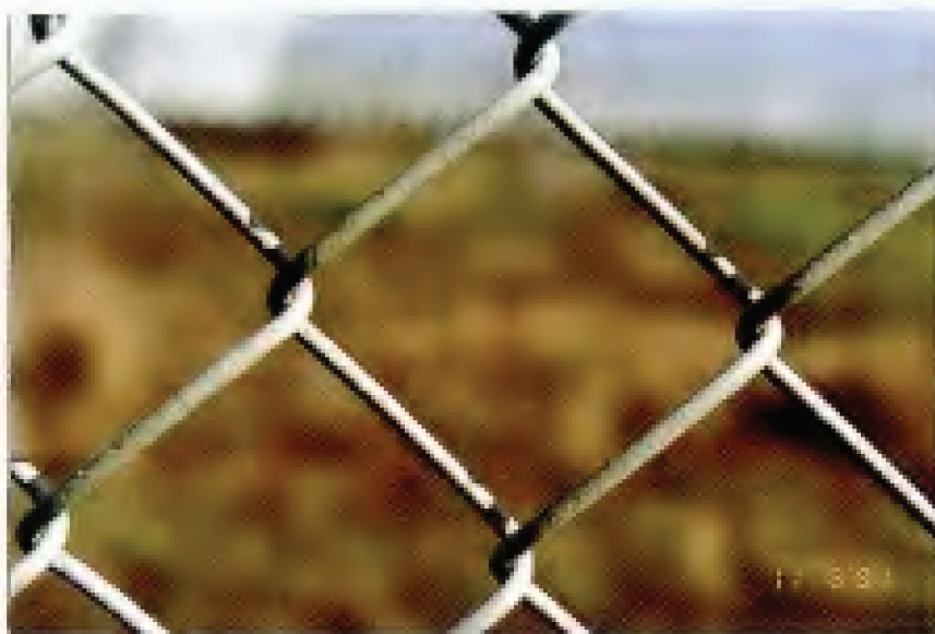
FIG. 36. Specimen 36 – Hot-Dip Aluminized Chain Link Fabric. Original coating weight: 0.57 oz/ft 2 (174 g/m 2 ). Exposure site: Point Reyes, CA. 30-year condition of links (see Table 13): 50M, 50G.
