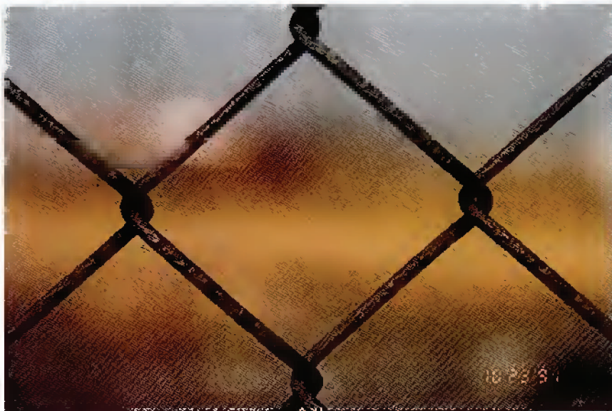
FIG. 21. Specimen 34 – Zinc Electroplated Chain Link Fabric. Original coating weight: 1.53 oz/ft 2 (467 g/m 2 ). Exposure site: Newark-Kearny, NJ. 30-year condition of links (see Table 13): 100R.
