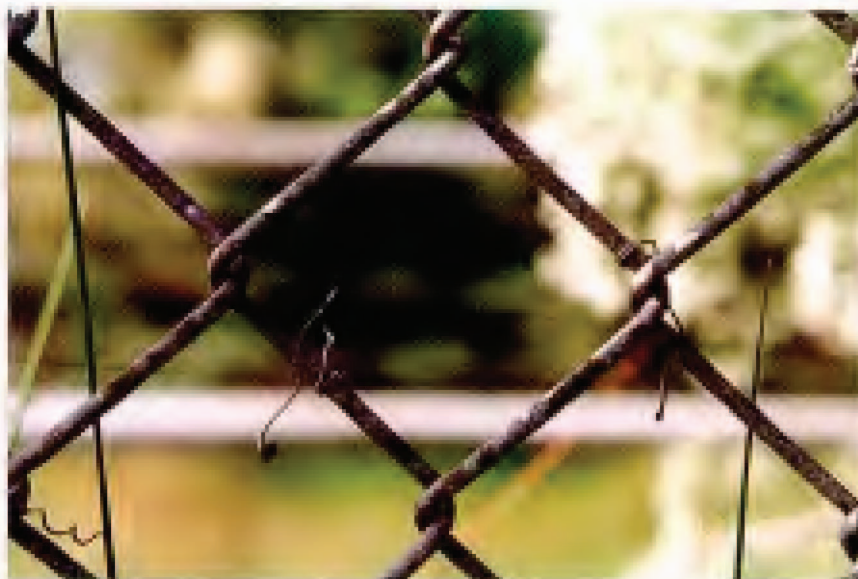
FIG. 46. Specimen 38 – Hot-Dip Aluminized Chain Link Fabric. Original coating weight: 0.54 oz/ft 2 (165 g/m 2 ). Exposure site: Brazos River, TX. 30-year condition of links (see Table 13): 5R, 20wc, 75G.
