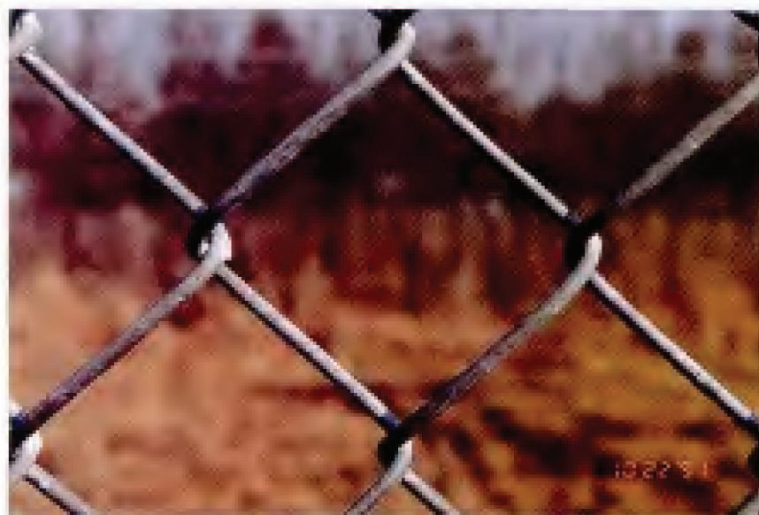
FIG. 7. Specimen 32 – Hot-dip Galvanized Chain Link Fabric. Original coating weight: 1.77 oz/ft 2 (540 g/m 2 ). Exposure site: Manhattan, KS. 30-year condition of links (see Table 13): 40G, 60Y.
