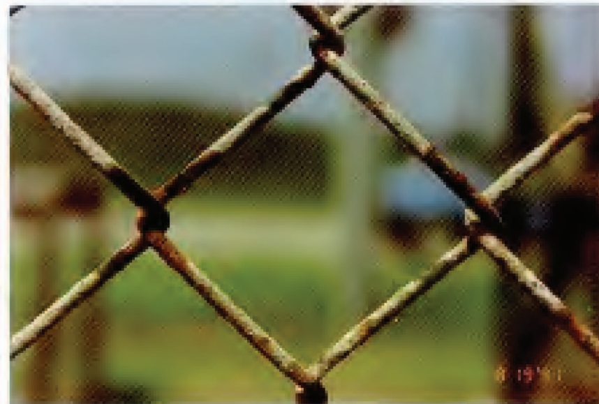
FIG. 12. Specimen 33 – Hot-dip Galvanized Chain Link Fabric. Original coating weight: 2.81 oz/ft 2 (857 g/m 2 ). Exposure site: Kure Beach, NC (80-ft site). 30-year condition of links (see Table 13): 95R, 5wc.
