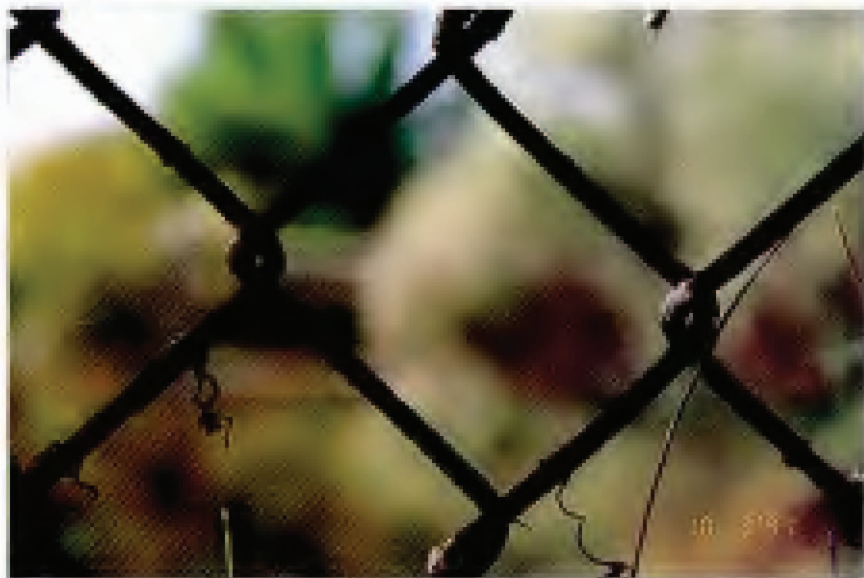
FIG. 4. Specimen 32 – Hot-dip Galvanized Chain Link Fabric. Original coating weight: 1.77 oz/ft 2 (540 g/m 2 ). Exposure site: Brazos River, TX. 30-year condition of links (see Table 13): 95R, 5wc.
