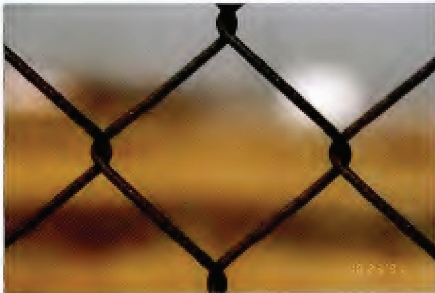
FIG. 42. Specimen 37 – Hot-Dip Aluminized Chain Link Fabric. Original coating weight: 0.44 oz/ft 2 (134 g/m 2 ). Exposure site: Newark-Kearny, NJ. 30-year condition of links (see Table 13): 10PPR, 90blk.
