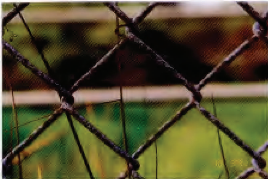
FIG. 24. Specimen 35 – Zinc Electroplated Chain Link Fabric. Original coating weight: 2.23 oz/ft 2 (680 g/m 2 ). Exposure site: Brazos River, TX. 30-year condition of links (see Table 13): 15R, 85wc.
