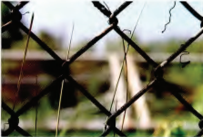
FIG. 30. Specimen 36 – Hot-Dip Aluminized Chain Link Fabric. Original coating weight: 0.57 oz/ft 2 (174 g/m 2 ). Exposure site: Brazos River, TX. 30-year condition of links (see Table 13): 10R, 15wc, 75G.
