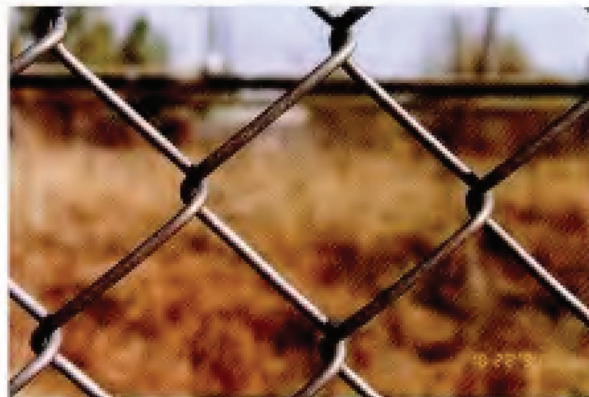
FIG. 49. Specimen 38 – Hot-Dip Aluminized Chain Link Fabric. Original coating weight: 0.54 oz/ft 2 (165 g/m 2 ). Exposure site: Manhattan, KS. 30-year condition of links (see Table 13): 50M, 50st.
