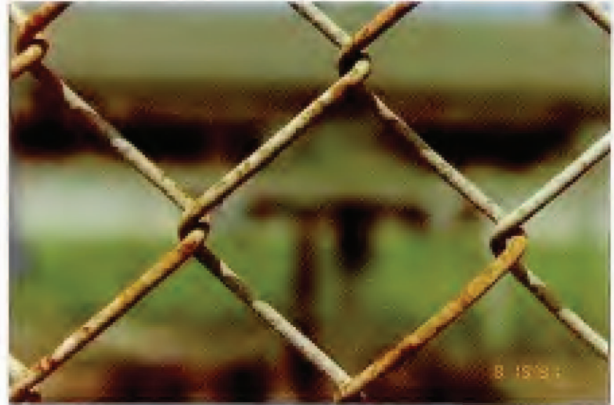
FIG. 31. Specimen 36 – Hot-Dip Aluminized Chain Link Fabric. Original coating weight: 0.57 oz/ft 2 (174 g/m 2 ). Exposure site: Kure Beach, NC (80-ft site). 30-year condition of links (see Table 13): 30R, 20Y, 50G, trM.
