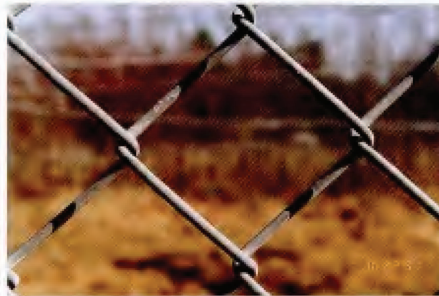
FIG. 14. Specimen 33 – Hot-dip Galvanized Chain Link Fabric. Original coating weight: 2.81 oz/ft 2 (857 g/m 2 ). Exposure site: Manhattan, KS. 30-year condition of links (see Table 13): 40G, 60Y.
