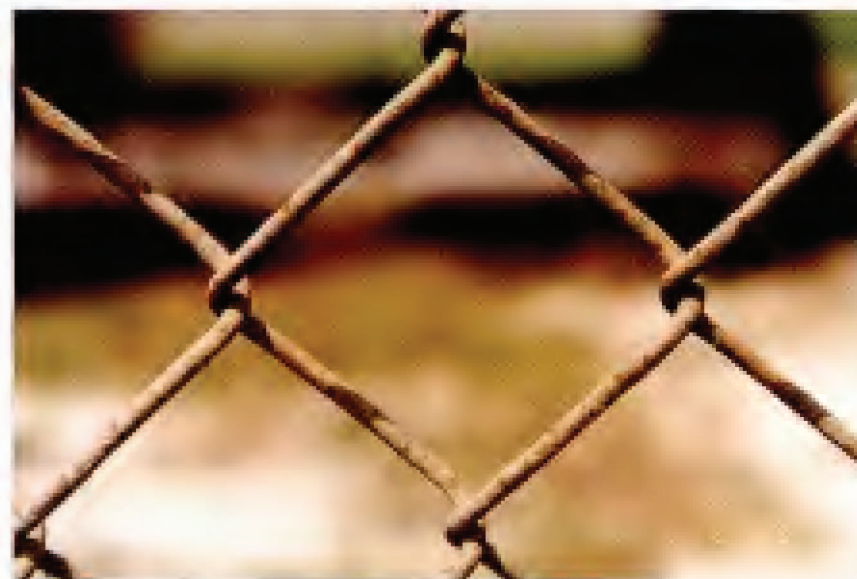
FIG. 47. Specimen 38 – Hot-Dip Aluminized Chain Link Fabric. Original coating weight: 0.54 oz/ft 2 (165 g/m 2 ). Exposure site: Kure Beach, NC (80-ft site). 30-year condition of links (see Table 13): 50R, 25Y, 25G.
