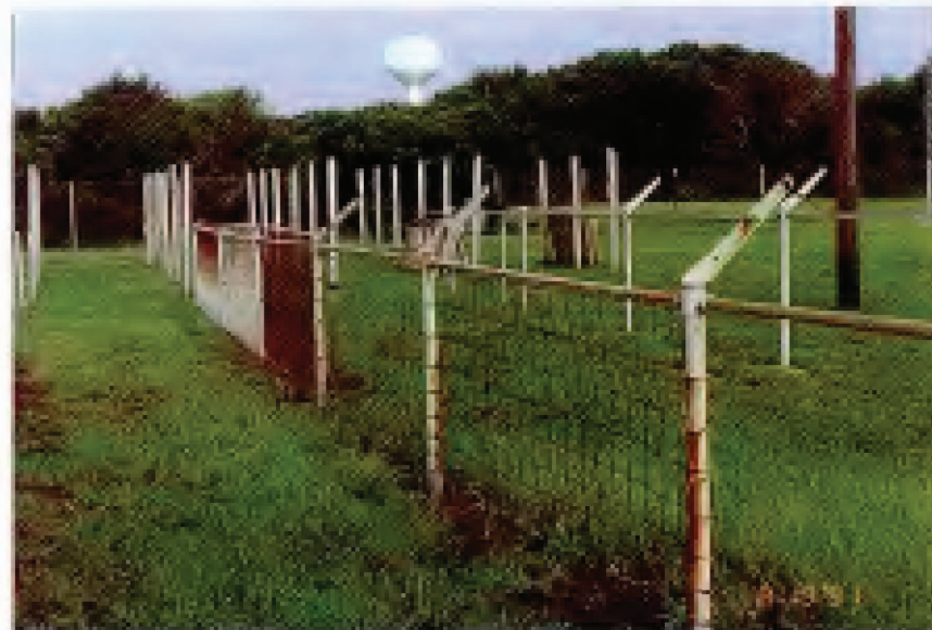
FIG. 2. Overall View of the Kure Beach, NC 800-ft Test Site illustrates the mounting of the field fence, barbed wire, and chain link fabric test specimens.
