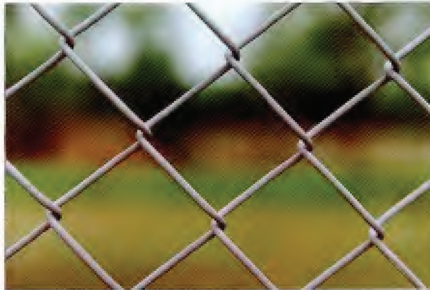
FIG. 29. Specimen 35 – Zinc Electroplated Chain Link Fabric. Original coating weight: 2.23 oz/ft 2 (680 g/m 2 ). Exposure site: State College, PA. 30-year condition of links (see Table 13): 100G.
