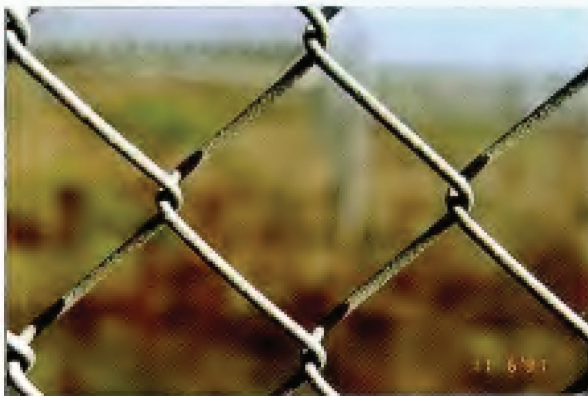
FIG. 44. Specimen 37 – Hot-Dip Aluminized Chain Link Fabric. Original coating weight: 0.44 oz/ft 2 (134 g/m 2 ). Exposure site: Point Reyes, CA. 30-year condition of links (see Table 13): 1PPR, 99wc.
