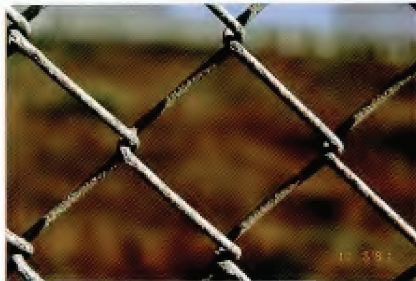
FIG. 16. Specimen 33 – Hot-dip Galvanized Chain Link Fabric. Original coating weight: 2.81 oz/ft 2 (857 g/m 2 ). Exposure site: Point Reyes, CA. 30-year condition of links (see Table 13): 5PPR, 95wc.
