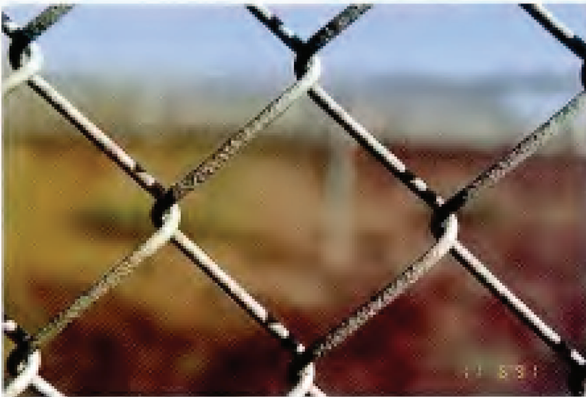
FIG. 52. Specimen 38 – Hot-Dip Aluminized Chain Link Fabric. Original coating weight: 0.54 oz/ft 2 (165 g/m 2 ). Exposure site: Point Reyes, CA. 30-year condition of links (see Table 13): 5PPR, 95wc.
