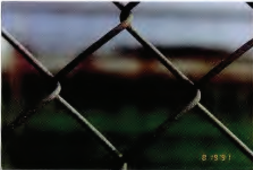
FIG. 32. Specimen 36 – Hot-Dip Aluminized Chain Link Fabric. Original coating weight: 0.57 oz/ft 2 (174 g/m 2 ). Exposure site: Kure Beach, NC (800-ft site). 30-year condition of links (see Table 13): 2R, 10wc, 78G, 10M.
