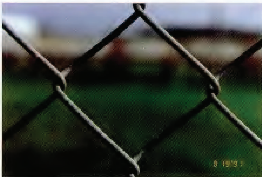
FIG. 40. Specimen 37 – Hot-Dip Aluminized Chain Link Fabric. Original coating weight: 0.44 oz/ft 2 (134 g/m 2 ). Exposure site: Kure Beach, NC (800-ft site). 30-year condition of links (see Table 13): 1R, 20wc, 74G, 5M.
