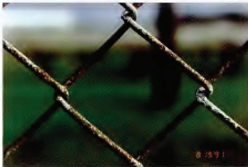
FIG. 13. Specimen 33 – Hot-dip Galvanized Chain Link Fabric. Original coating weight: 2.81 oz/ft 2 (857 g/m 2 ). Exposure site: Kure Beach, NC (800-ft site). 30-year condition of links (see Table 13): 40R, 60wc.
