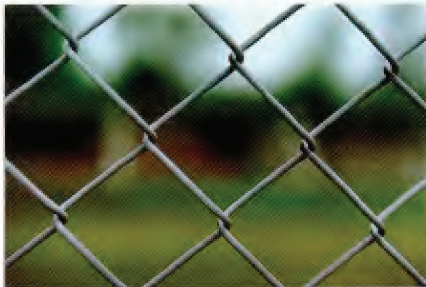
FIG. 23. Specimen 34 – Zinc Electroplated Chain Link Fabric. Original coating weight: 1.53 oz/ft 2 (467 g/m 2 ). Exposure site: State College, PA. 30-year condition of links (see Table 13): 100G.
