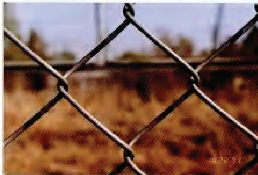
FIG. 41. Specimen 37 – Hot-Dip Aluminized Chain Link Fabric. Original coating weight: 0.44 oz/ft 2 (134 g/m 2 ). Exposure site: Manhattan, KS. 30-year condition of links (see Table 13): 40M, 60st.
