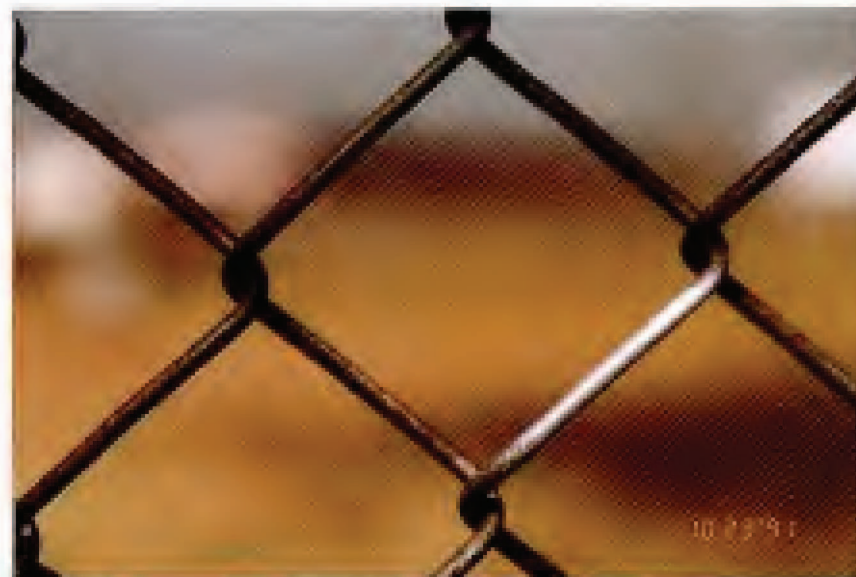
FIG. 35. Specimen 36 – Hot-Dip Aluminized Chain Link Fabric. Note: This is same specimen as illustrated in Fig. 34, with black corrosion product removed on one straight wire segment to illustrate that aluminum coating is still intact.
