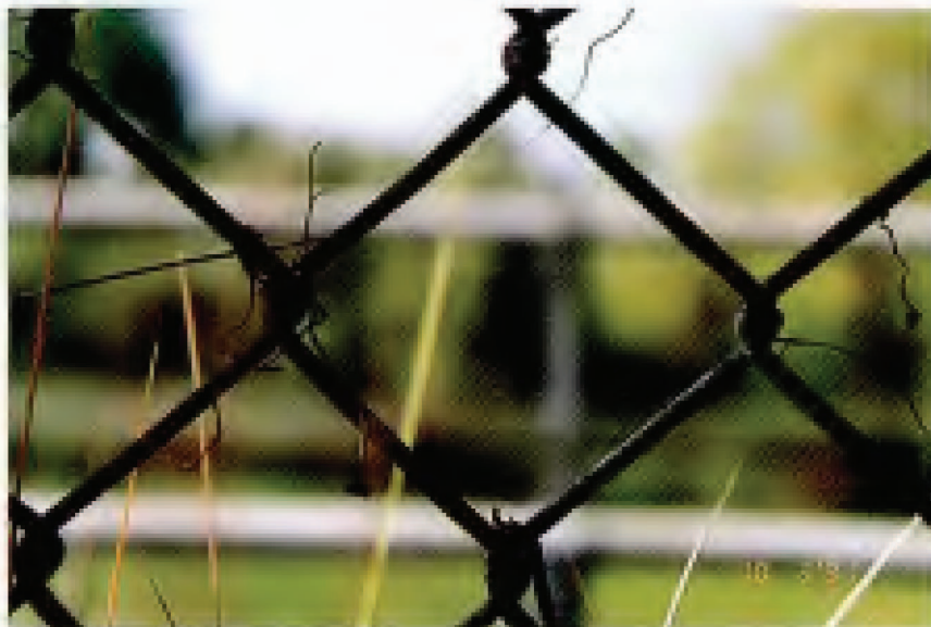
FIG. 38. Specimen 37 – Hot-Dip Aluminized Chain Link Fabric. Original coating weight: 0.44 oz/ft 2 (134 g/m 2 ). Exposure site: Brazos River, TX. 30-year condition of links (see Table 13): 15R, 75wc, 10G.
