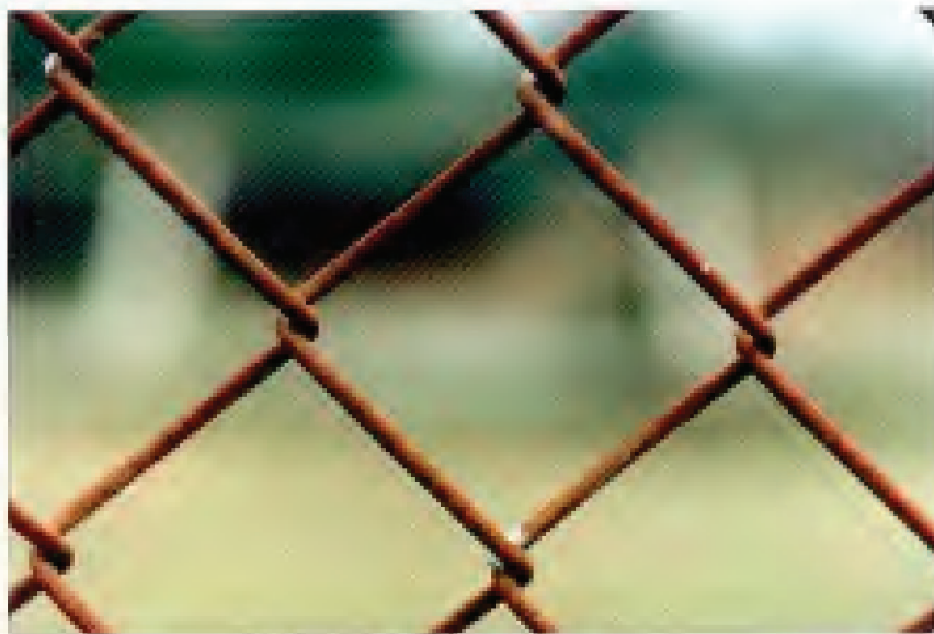
FIG. 17. Specimen 33 – Hot-dip Galvanized Chain Link Fabric. Original coating weight: 2.81 oz/ft 2 (857 g/m 2 ). Exposure site: State College, PA. 30-year condition of links (see Table 13): 5G, 95Y.
