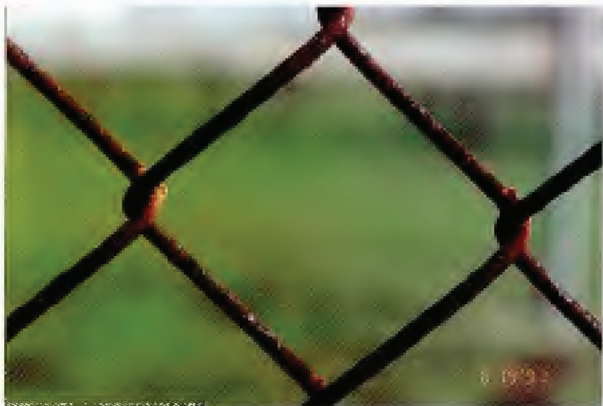
FIG. 6. Specimen 32 – Hot-dip Galvanized Chain Link Fabric. Original coating weight: 1.77 oz/ft 2 (540 g/m 2 ). Exposure site: Kure Beach, NC (800-ft site). 30-year condition of links (see Table 13): 95R, 5wc.
