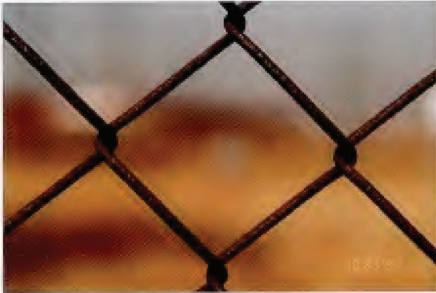
FIG. 27. Specimen 35 – Zinc Electroplated Chain Link Fabric. Original coating weight: 2.23 oz/ft 2 (680 g/m 2 ). Exposure site: Newark-Kearny, NJ. 30-year condition of links (see Table 13): 100R.
