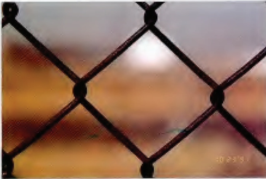
FIG. 50. Specimen 38 – Hot-Dip Aluminized Chain Link Fabric. Original coating weight: 0.54 oz/ft 2 (165 g/m 2 ). Exposure site: Newark-Kearny, NJ. 30-year condition of links (see Table 13): 10PPR, 90 blk.
