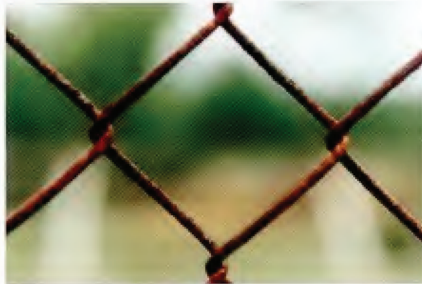
FIG. 10. Specimen 32 – Hot-dip Galvanized Chain Link Fabric. Original coating weight: 1.77 oz/ft 2 (540 g/m 2 ). Exposure site: State College, PA. 30-year condition of links (see Table 13): 95R, 5Y.
