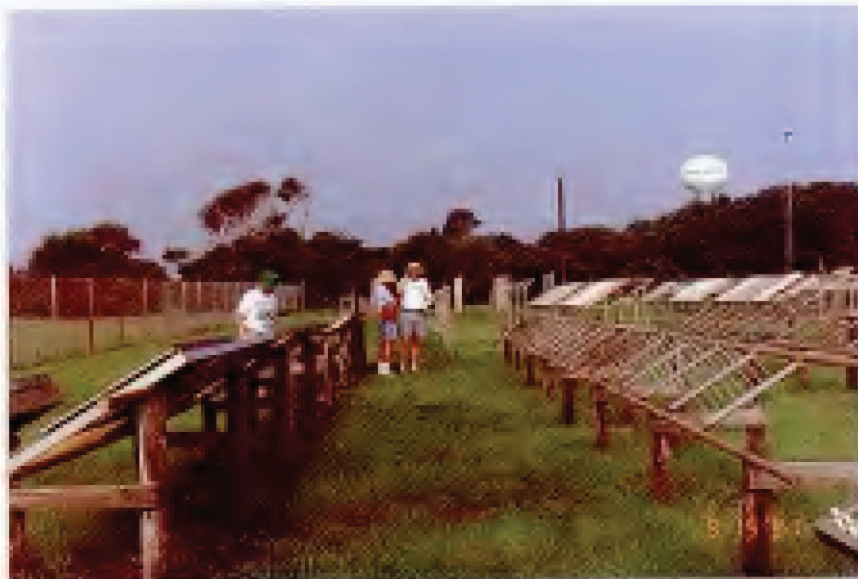
FIG. 1. Overall View of the Kure Beach, NC 800-ft Test Site illustrates the mounting of the unfabricated test wire specimens.
