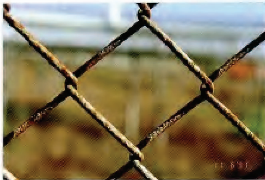
FIG. 22. Specimen 34 – Zinc Electroplated Chain Link Fabric. Original coating weight: 1.53 oz/ft 2 (467 g/m 2 ). Exposure site: Point Reyes, CA. 30-year condition of links (see Table 13): 50R, 20wc, 30G.
