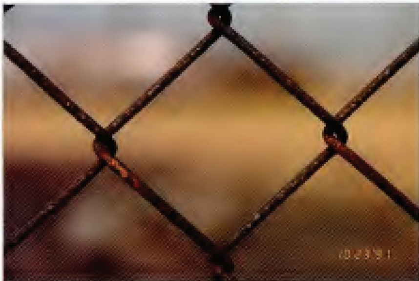
FIG. 15. Specimen 33 – Hot-dip Galvanized Chain Link Fabric. Original coating weight: 2.81 oz/ft 2 (857 g/m 2 ). Exposure site: Newark-Kearny, NJ. 30-year condition of links (see Table 13): 100R.
