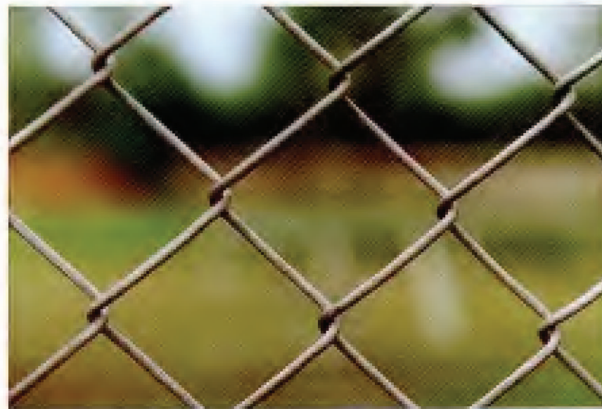
FIG. 37. Specimen 36 – Hot-Dip Aluminized Chain Link Fabric. Original coating weight: 0.57 oz/ft 2 (174 g/m 2 ). Exposure site: State College, PA. 30-year condition of links (see Table 13): 100G.
