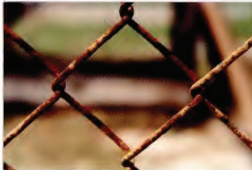
FIG. 39. Specimen 37 – Hot-Dip Aluminized Chain Link Fabric. Original coating weight: 0.44 oz/ft 2 (134 g/m 2 ). Exposure site: Kure Beach, NC (80-ft site). 30-year condition of links (see Table 13): 55R, 25Y, 20G.
