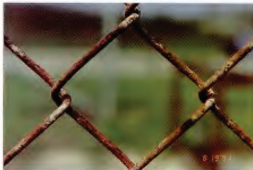
FIG. 5. Specimen 32 – Hot-dip Galvanized Chain Link Fabric. Original coating weight: 1.77 oz/ft 2 (540 g/m 2 ). Exposure site: Kure Beach, NC (80-ft site). 30-year condition of links (see Table 13): 100R.
