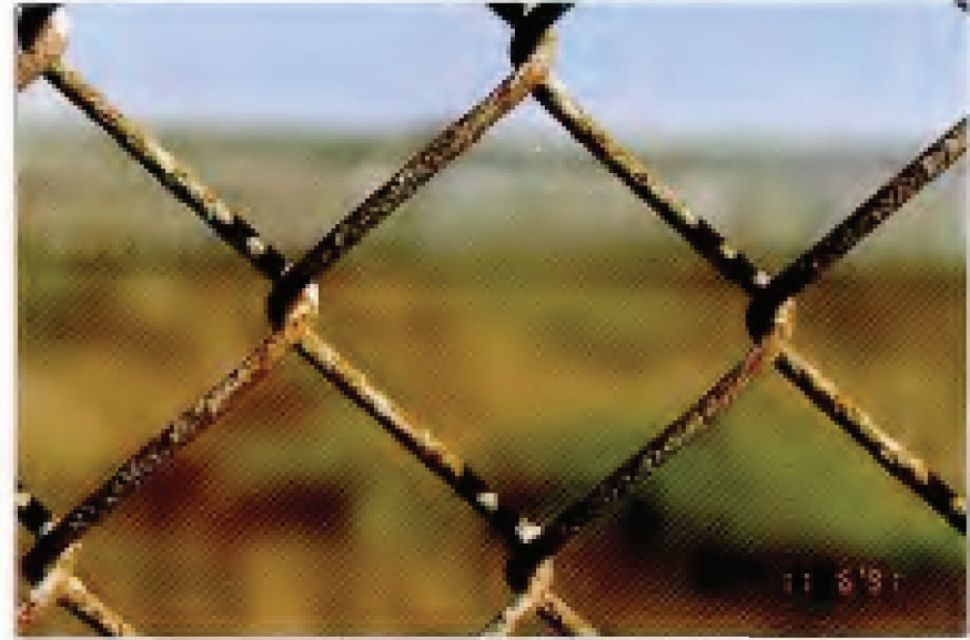
FIG. 9. Specimen 32 – Hot-dip Galvanized Chain Link Fabric. Original coating weight: 1.77 oz/ft 2 (540 g/m 2 ). Exposure site: Point Reyes, CA. 30-year condition of links (see Table 13): 60R, 40wc.
