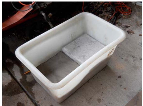
FIG. X1.5 Additional Porous Stones Are Used as Confining Pressure
