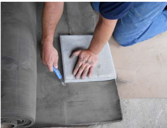
FIG. X1.3 Coupons 300 by 300 mm [12 by 12 in.] Are Cut from Roll
