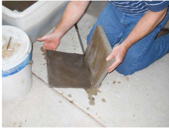
FIG. X1.8 Separate Coupon from Porous Stone GM Side Does Not Stick GT Side Does
