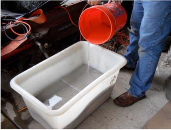
FIG. X1.6 Tub is Flooded and Allowed to Cure for 24 h
