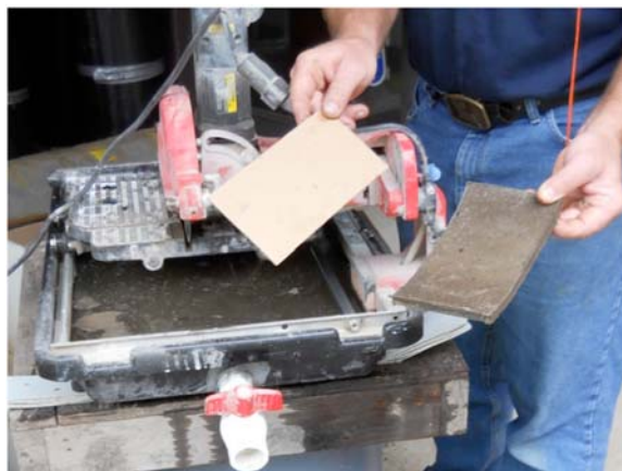
FIG. X1.10 Wet Diamond Saw Cutting of Specimen from Coupon
