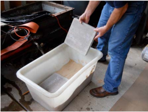
FIG. X1.2 Porous Stones 300 by 300 mm [12 by 12 in.] Placed on Leveling Sand
