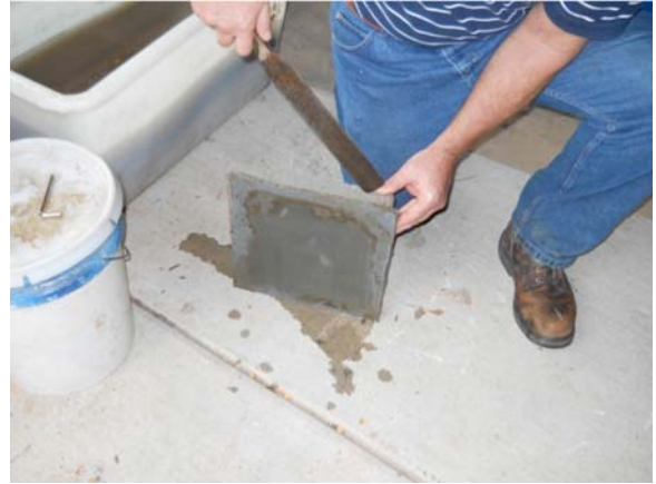
FIG. X1.7 With Large Flat Knife Cured Sample is Stripped Away from Porous Stone
