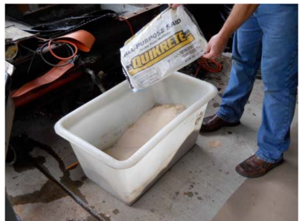
FIG. X1.1 Sand Placed in Base of Tub
