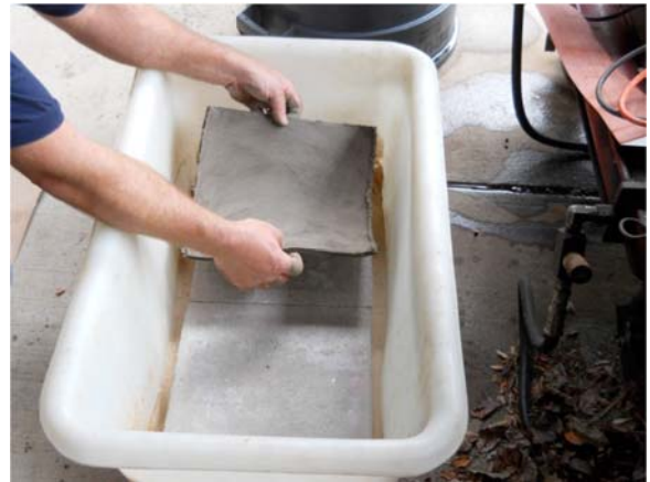
FIG. X1.4 Coupons Are Placed on Top of Porous Stones
