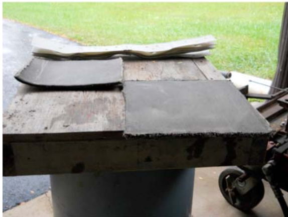
FIG. X1.9 Comparison of Free Swell and Confined Swell Coupons
