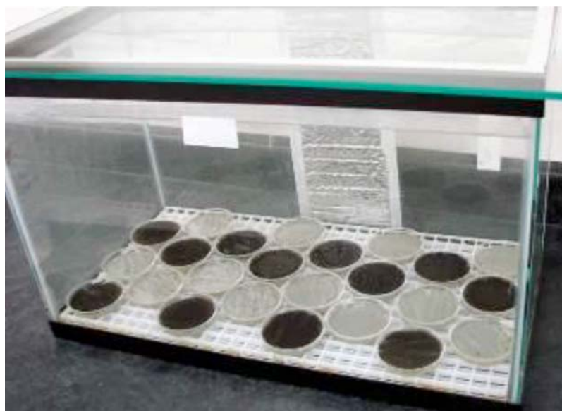
FIG. 4 Example of Sporulating Fungal Plates Arranged in an Alternating Pattern in the Environmental Chamber
