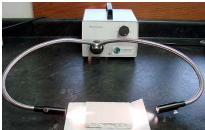
FIG. 5 Light Pipes Illuminating Surface of Test Specimen
