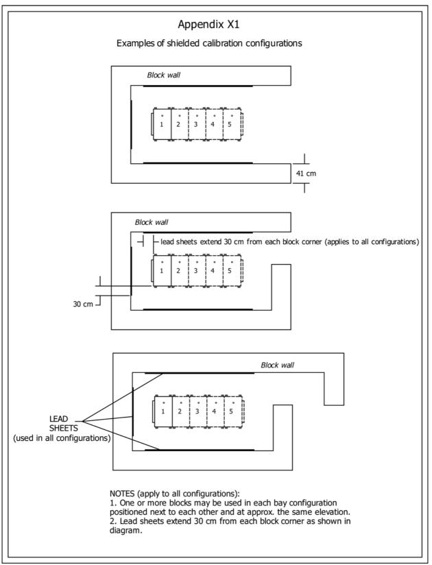
FIG. X1.1 Three different shielded calibration and storage bay configurations
