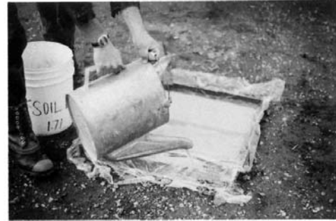
FIG. 4 Sand Being Poured Into the Template
