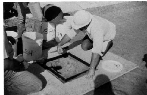
FIG. 5 Excavation of the Test Pit
