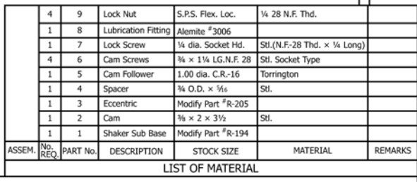
FIG. 2 Modification of Tyler Portable Sieve Shaker
