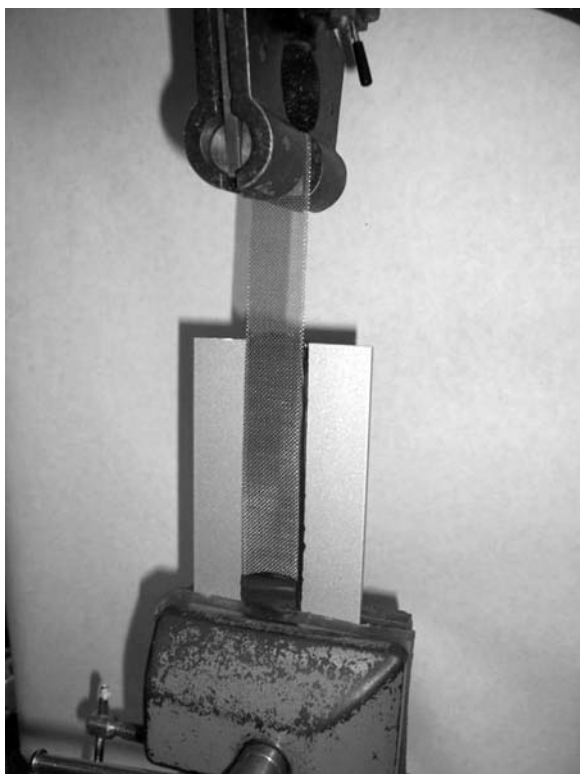
FIG. 10 Adhesion-in-Peel Test Specimen Secured in Tensile Testing Machine
