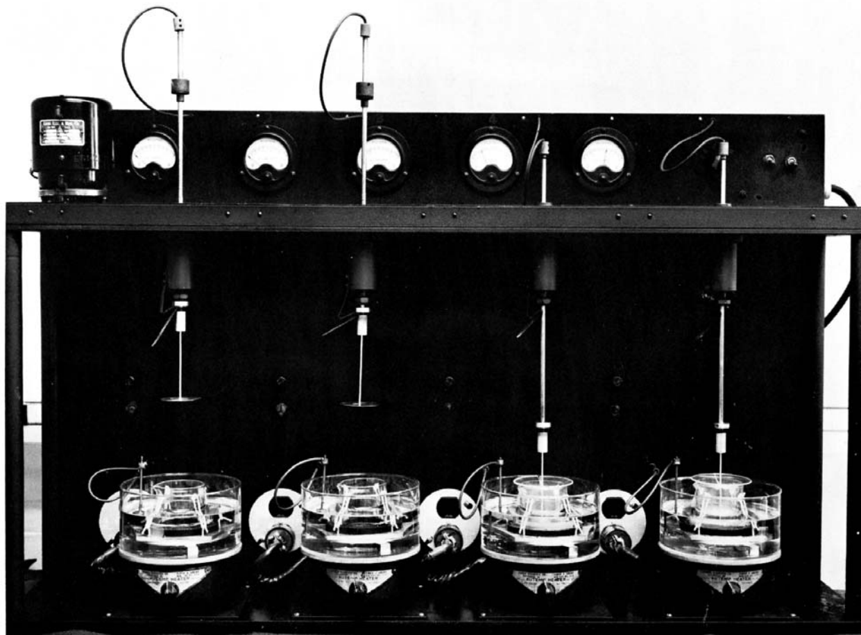
FIG. 4 Multiple-Cell Electroplating Apparatus
