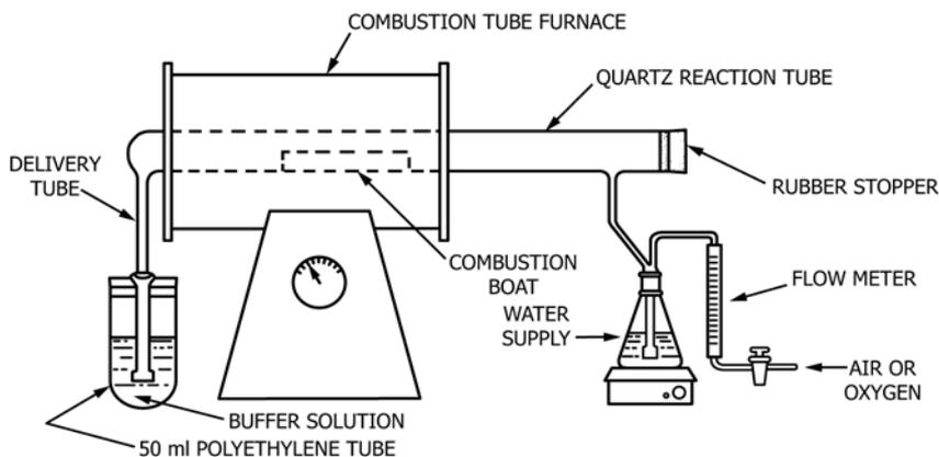
FIG. 3 Pyrohydrolysis Apparatus
