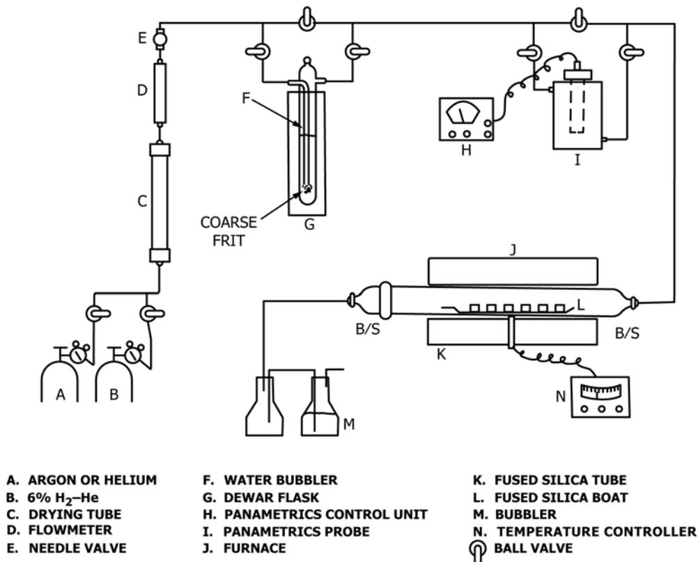
FIG. 6 O/M Apparatus
