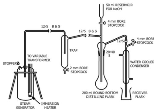
FIG. 1 Distillation Apparatus
