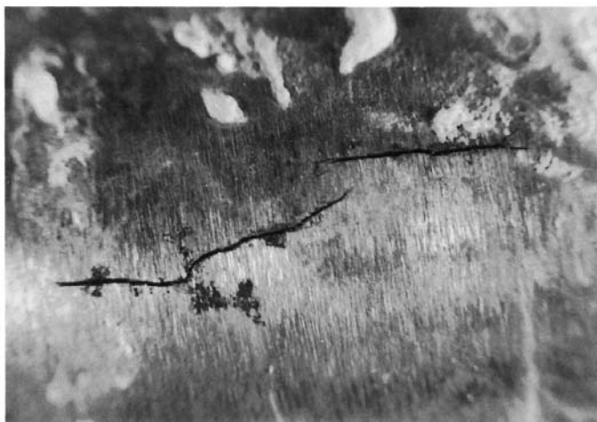
FIG. 2 Typical External Stress Corrosion Cracks (5× Magnification)
