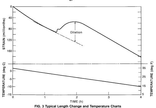
by measuring the vertical distance from a straightline projection of the prefreezing, length- *versus*-time contraction curve (at constant cooling rate) and the maximum deviation of the strain trace from it (Fig. 3).
