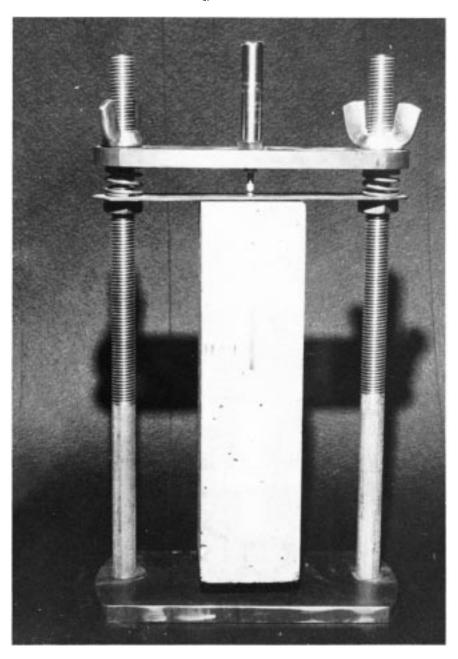
Note 1—The drawings in Adjunct C 671 show an experimental setup slightly different from this one. FIG. 1 Specimen Positioned in Strain Frame
