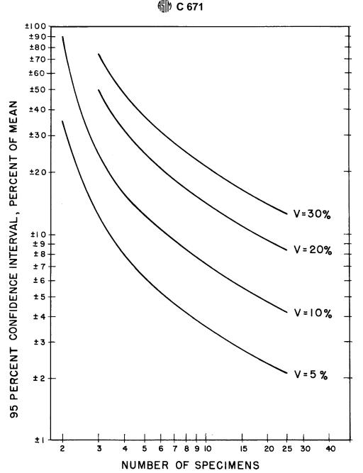
FIG. 4 Ninety-five Percent Confidence Interval Versus Number of Specimens for Determination of the Period of Frost Immunity<sup>6</sup>
