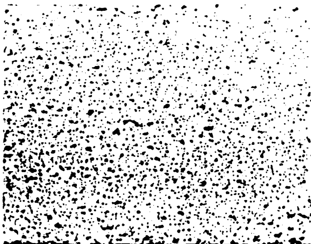
FIG. 1 Reboiling of Porcelain Enamel on Steel
