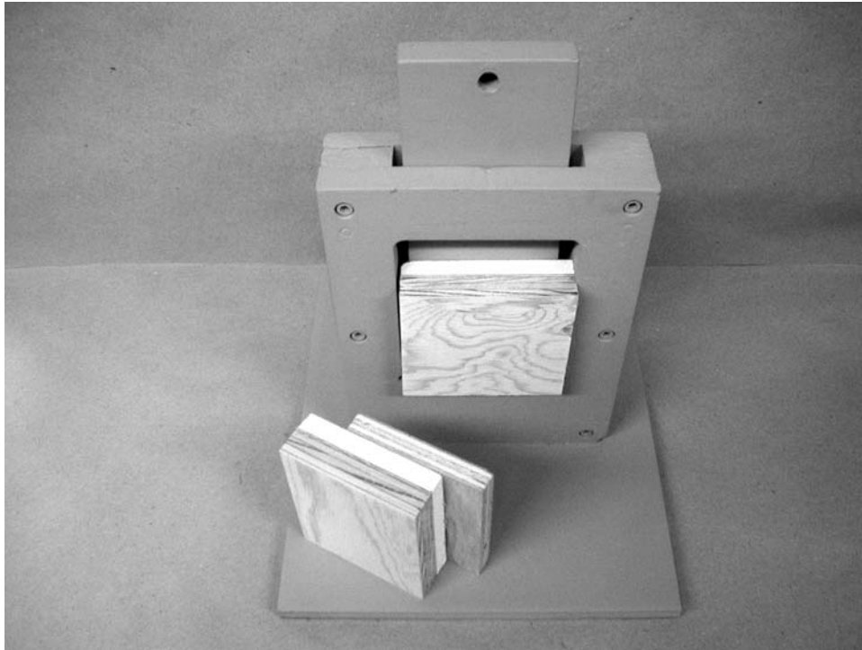
FIG. 1 Shear Strength Test Specimen in Text Fixture
