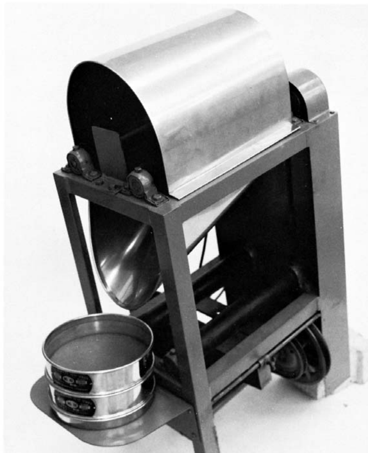
FIG. 3 Steel Jar Mill with Hood and Trough
