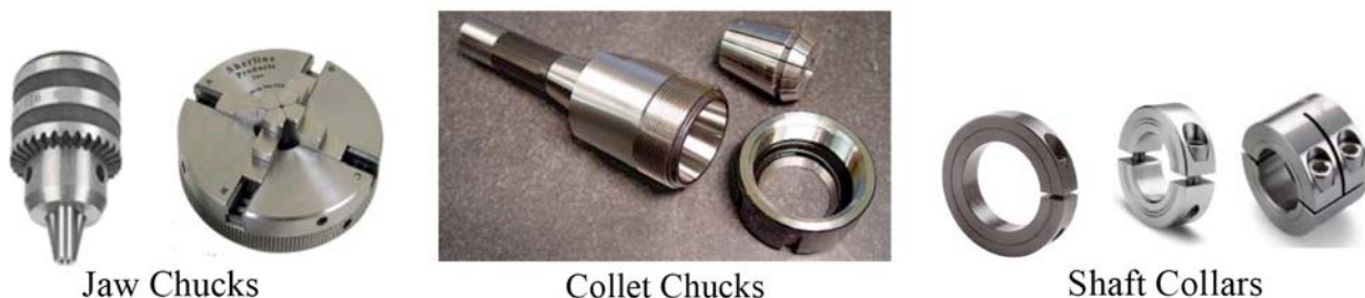
FIG. X2.1 Mechanical Grip Devices for the EPPO Test
