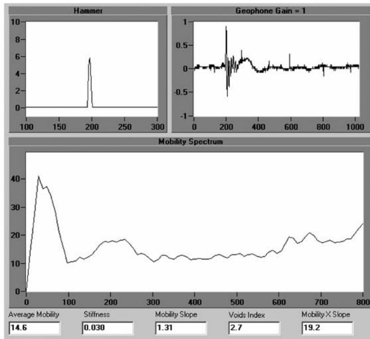
FIG. 5 Invalid Waveform (Upper Right Plot) Caused by Movement of the Velocity Transducer Base
