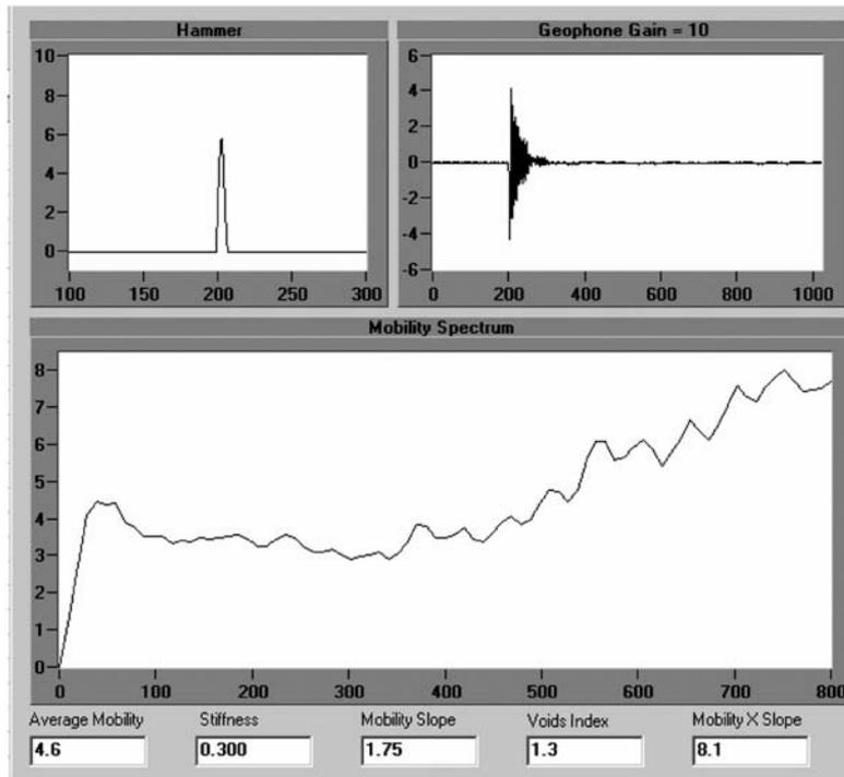
FIG. 4 Valid Set of Waveforms for Hammer Voltage Versus Time and Velocity Transducer Voltage Versus Time (Mobility Spectrum is at Bottom)
