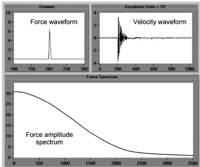
FIG. 2 Typical Force-Time Waveform and Amplitude Spectrum Plots for Hammer with a Hard Rubber Tip
