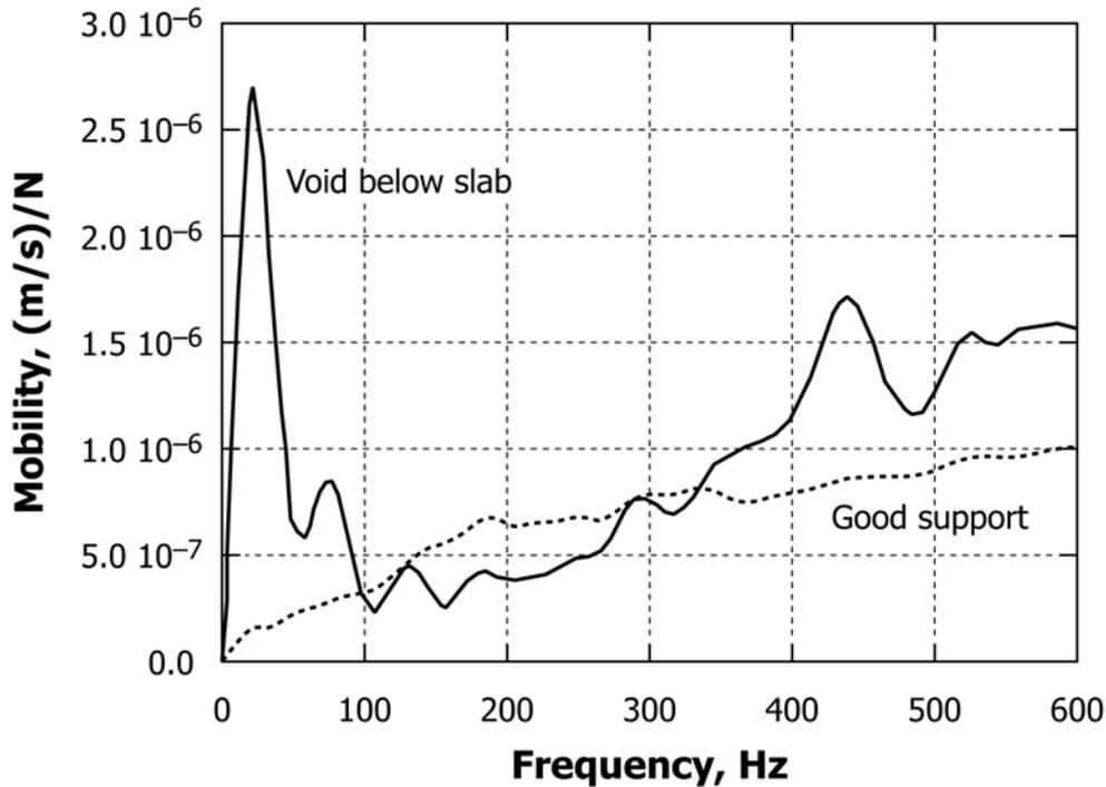
FIG. X1.3 Example of Mobility Spectrum for Test on Slab-on-Ground with Void Below Slab Compared with Test at Point Without Void
