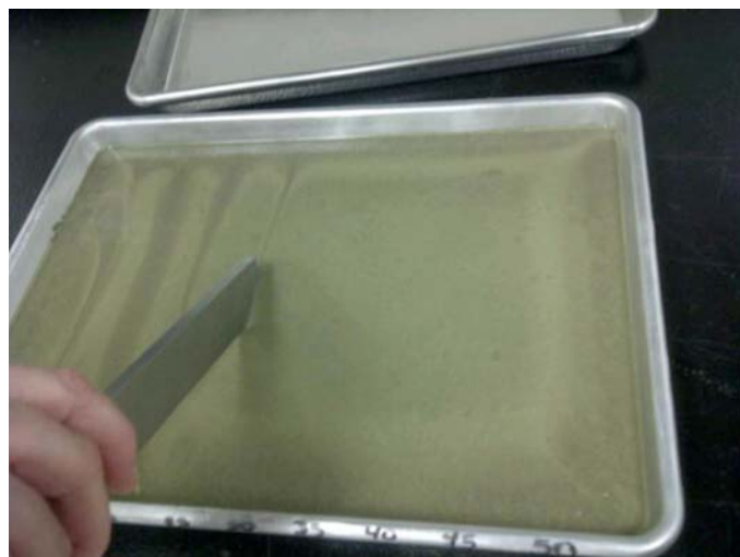
FIG. 1 Full-Depth Cut in Test Specimen
