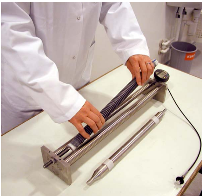
FIG. 9 Placement of Specimen in the Dilatometer Bench for Length Measurement
