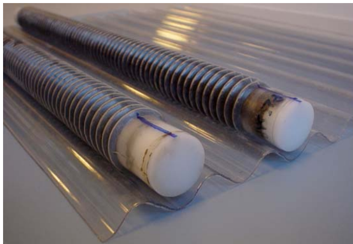
FIG. 8 Corrugated Plastic Sheets for Supporting the Specimens During the Test
