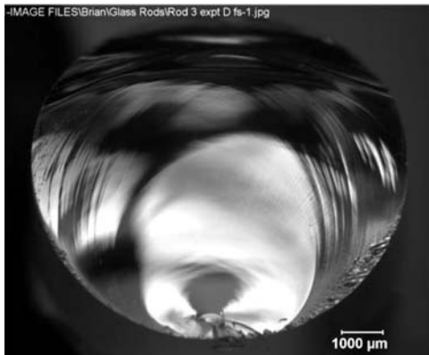
FIG. A3.4 Examples of Abnormal (Secondary) Fracture Surface in Glass Rods
