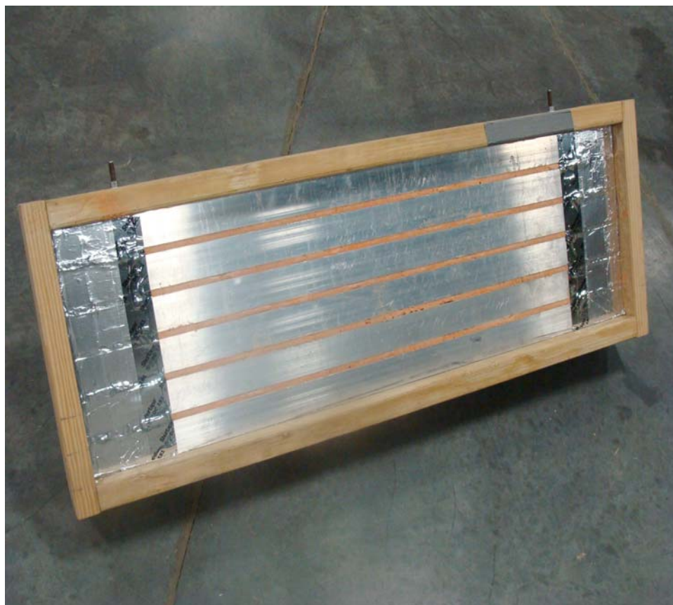
FIG. 2 Specimen Mounted into Wood Surround (test buck) – View from Interior Side.
