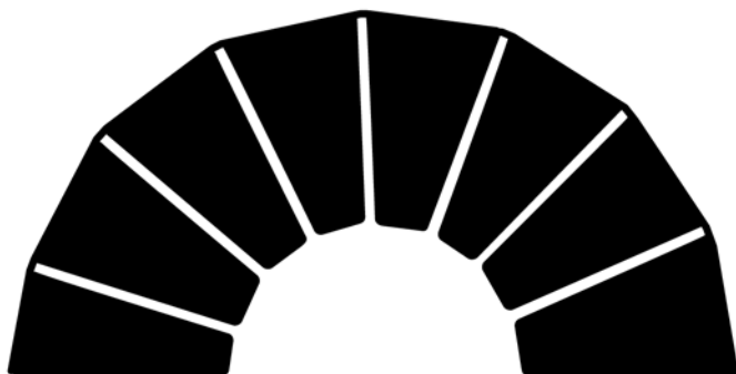
FIG. 6 Precision Cut V-Grooved Segmented Pipe Insulation
