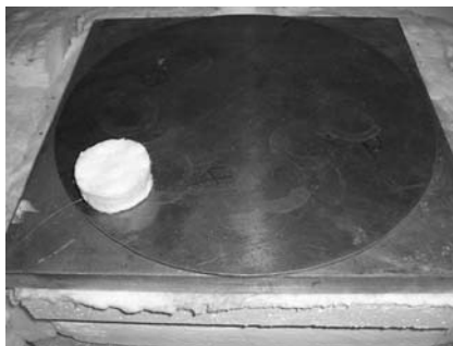
FIG. X1.1 A One-Foot Square Flat Plate Heater
