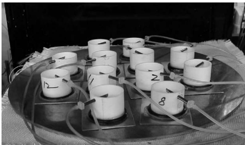
FIG. 3 Test Coupons on Hot Plate
