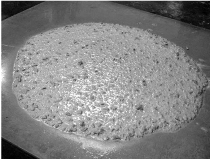
FIG. X1.2 VSI = 1 – Concrete Shows Slight Bleeding Observed as a Sheen on the Surface.
