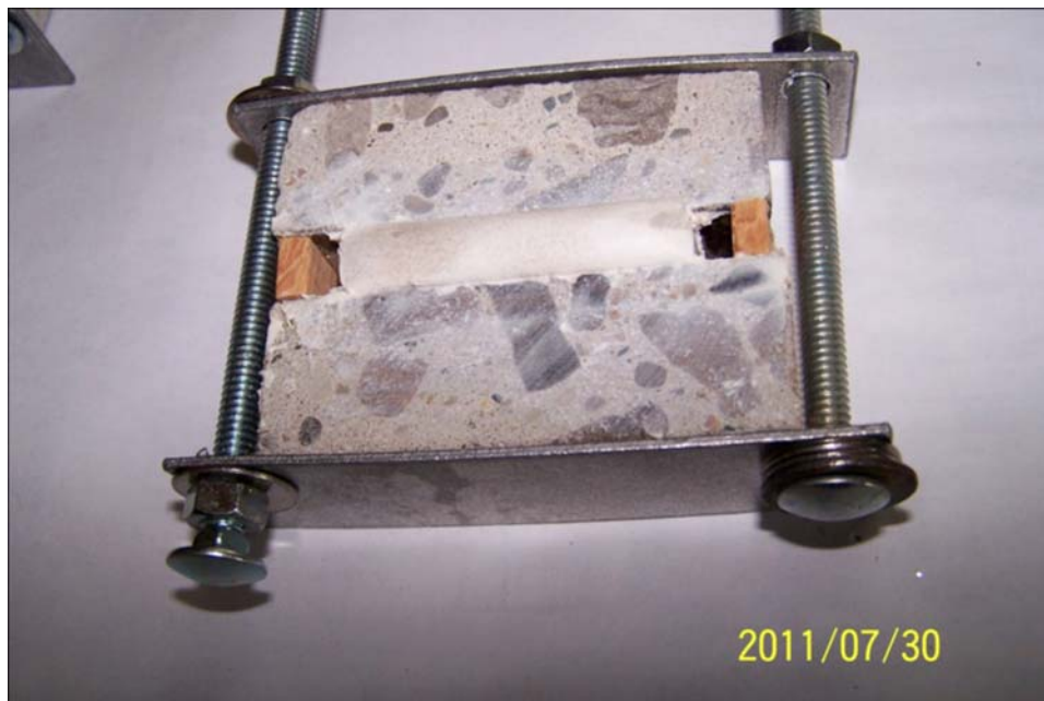
FIG. 3 Clamping Device Holding the Specimen in Compression
