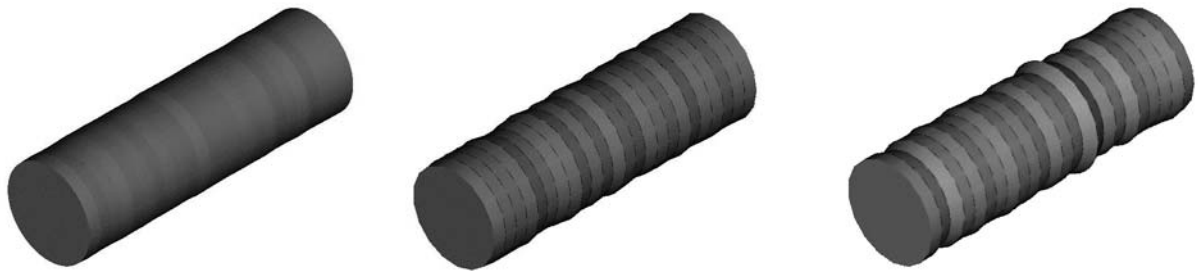
FIG. X1.2 Fiber Profiles Illustrating Variability of Fiber Diameter Along its Length
