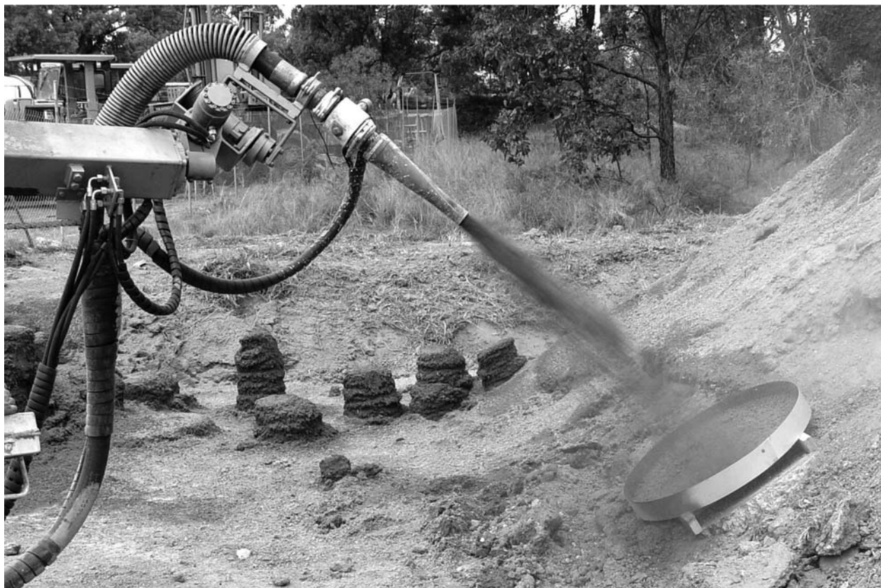
FIG. X1.6 Remotely-Controlled Spraying of Panels
