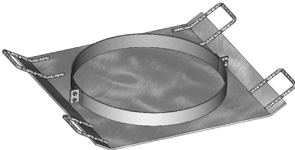
FIG. X1.2 Simple Steel Form With Rigid Base and Handles for Transport and Handling
