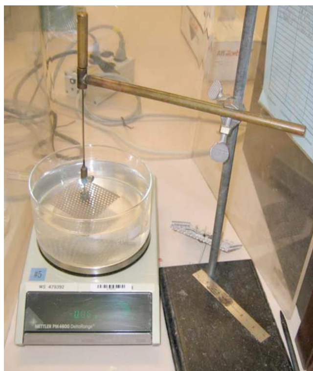
FIG. A1.2 Foam Beads In Cage Ready For Submersion In Water Tank
