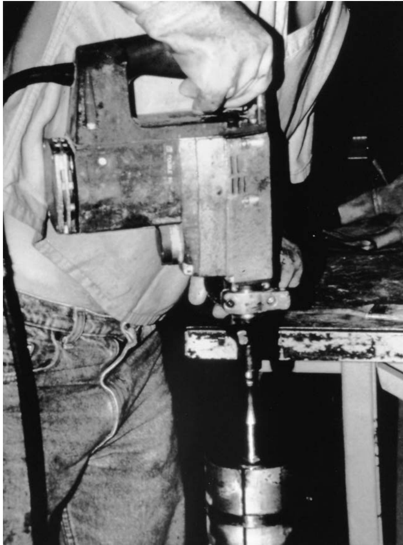
FIG. 1 Vibrating Hammer for Molding RCC Specimens
