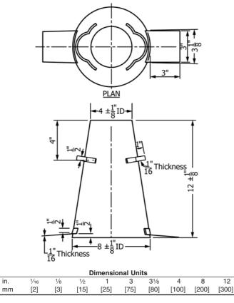
FIG. 1 Mold for Slump Test
