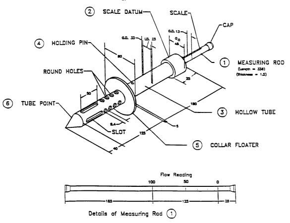
All dimensions in millimetres (1 in. = 25.4 mm) FIG. 1 Apparatus for Flow Test
