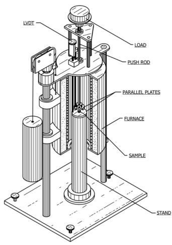
FIG. 1 A Typical Parallel Plate Viscometer
