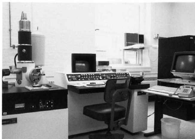
FIG. X4.3 Scanning Electron Microscope with Energy Dispersive Spectroscopic Capabilities, Low-Energy Operation, and Magnification Between 20 and 20 000×
