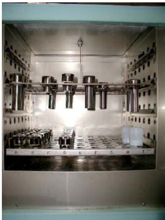
FIG. 2 Forced-air Circulation Blue M Oven with Numerous 304L Stainless Steel and Two Polytetrafluoroethylene Vessels.
