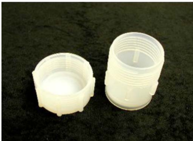
FIG. 1 (b) The 60 ml Polytetrafluoroethylene Vessel and Lid. The Vessels Should be Purchased with a Special Set of Plastic Wrenches (Not Shown) for Tightening. (continued)
