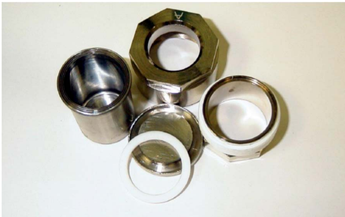
FIG. 1 (a) The Desensitized Type 304L Stainless Steel, 22 mL; PCT Vessel and Lid; a White Polytetrafluoroethylene Gasket Which Seals the Vessel and Lid When the Assembly is Closed and Tightened; and the Nickel-Plated Brass, Nut, and Screw Vessel Tightening Assembly.
