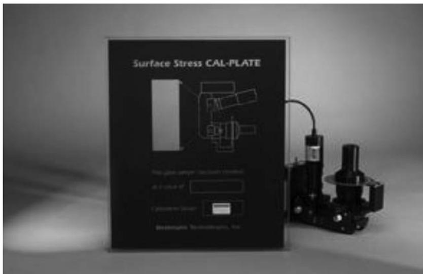
FIG. 8 Reference Standard (Cal-Plate) for Verifying Surface Polarimeters
