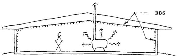
NOTE 1—Intended to protect inhabitants, materials and radiant heating or cooling sources from interior building surface temperature extremes.
