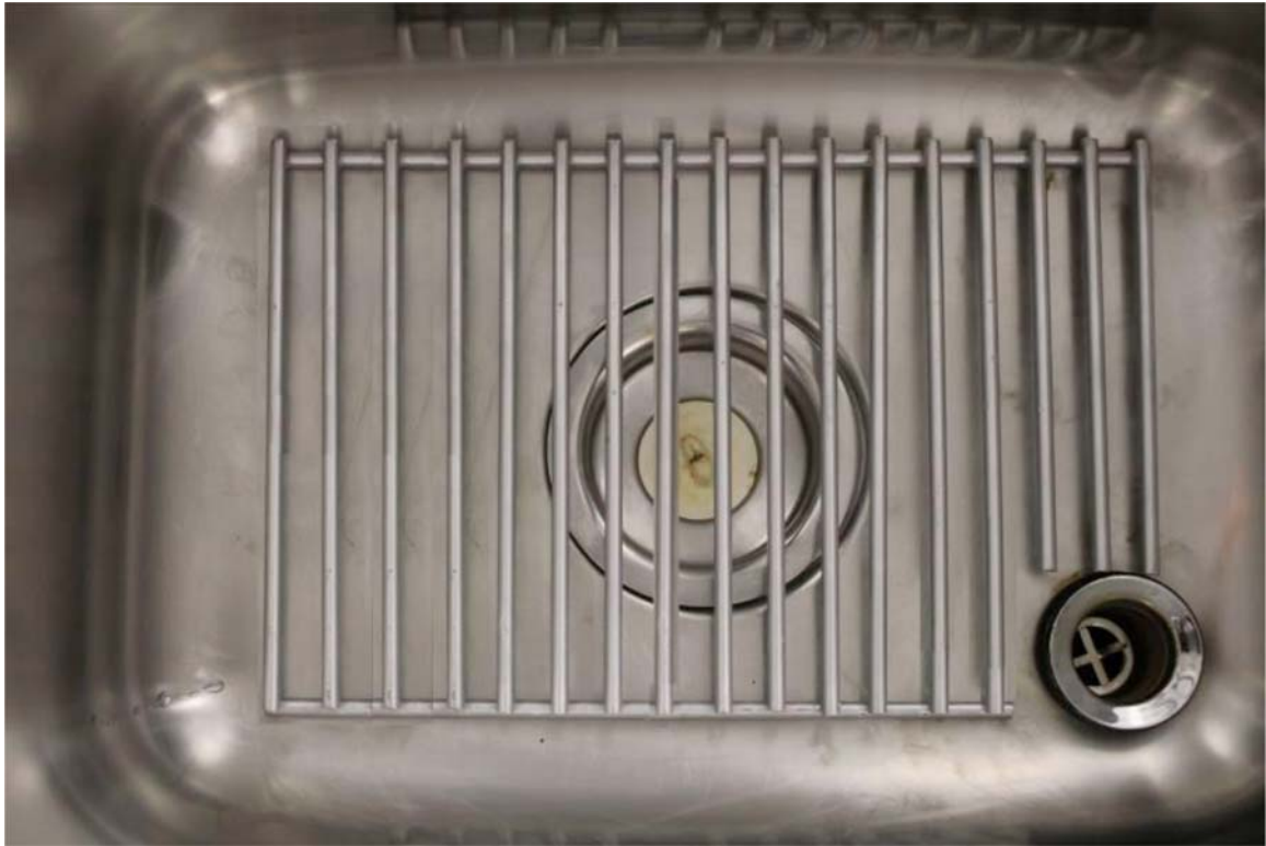
FIG. 4 Freezing Container with Tile Support Rack Installed
