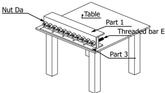
FIG. X1.9 Part 1 Engaged to Part 3, Part 3 Bolted to the Table
