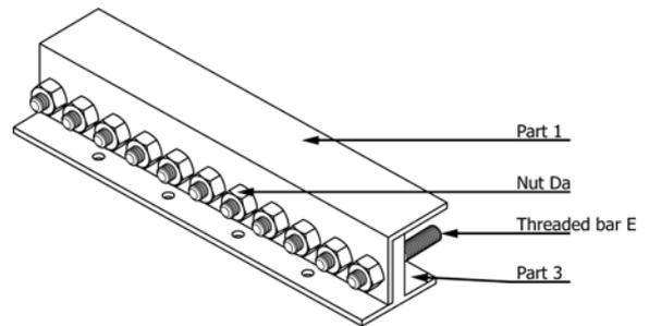
FIG. X1.6 Part 3 Coupled to Part 1
