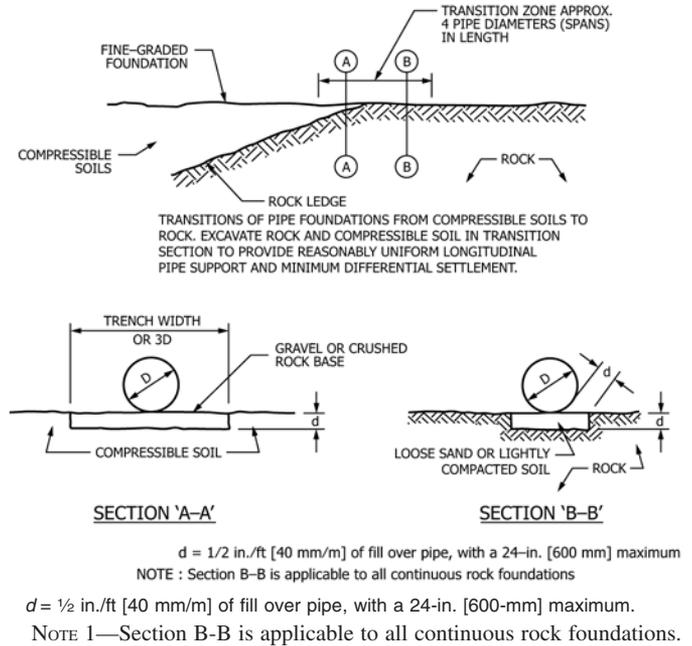
FIG. 3 Foundation Transition Zones and Rock Foundations
