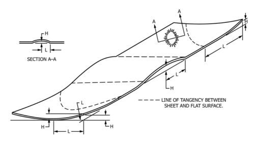
H = maximum distance between flat surface and lower surface of sheet.
