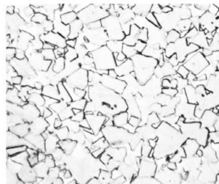
FIG. 2 Apparent Grain Size of Tungsten Carbide plus 10 % Cobalt (1500×)
