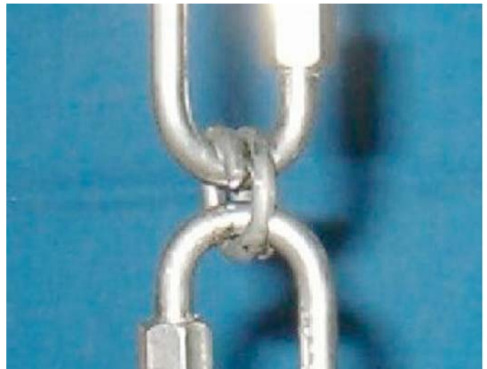
FIG. 5 Single Fastener Test with Load Applied Perpendicular to the Closing Axis
