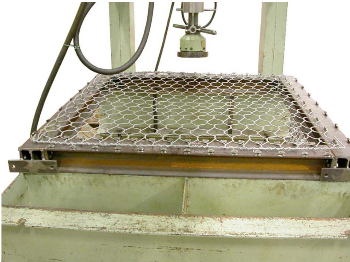
FIG. 6 Secured Punch Test with Every Mesh Clamped
