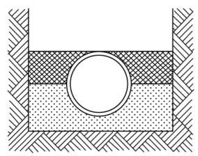
Note 1—Pipe is bedded to its centerline in compacted granular material with a minimum of 4 in. (102 mm) under the pipe. Compacted granular or select<sup>A</sup> material is used to the top of the pipe. (Material is compacted to approximately 90 % Standard Proctor in accordance with AASHTO Standard T-99.)
