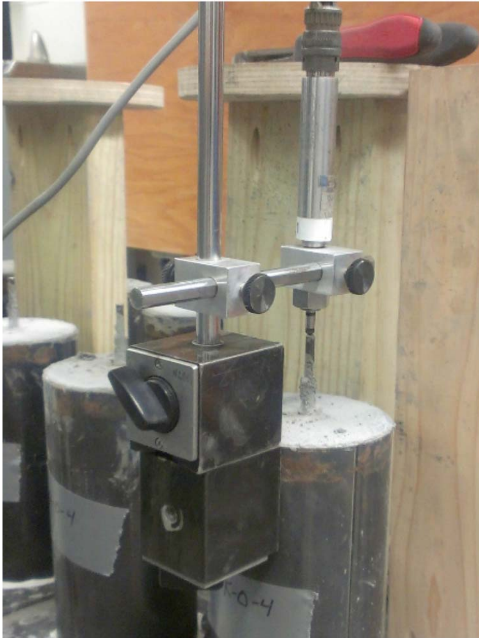
FIG. 4 LVDT and Magnetic Base Setup
