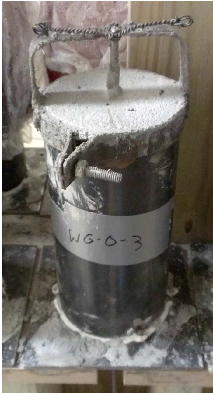
FIG. 3 Example of Fixture Used to Keep Wire Centered in Steel Casing During Mortar Placement and Consolidation
